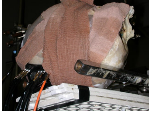
Figure 2.10: Human skull model filled with Intralipid solution. The lighter fiber is the source fiber and the 8 black fibers are the detector fibers. The skull is held inverted, filled with Intralipid. The probe is secured tightly to the skull with elastic bandage.
