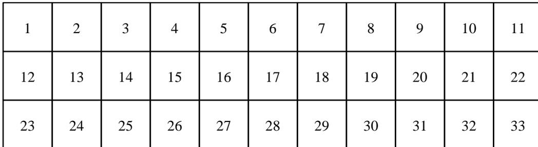
Figure 2.11: Arrangement of Macro Blocks in a GOB
