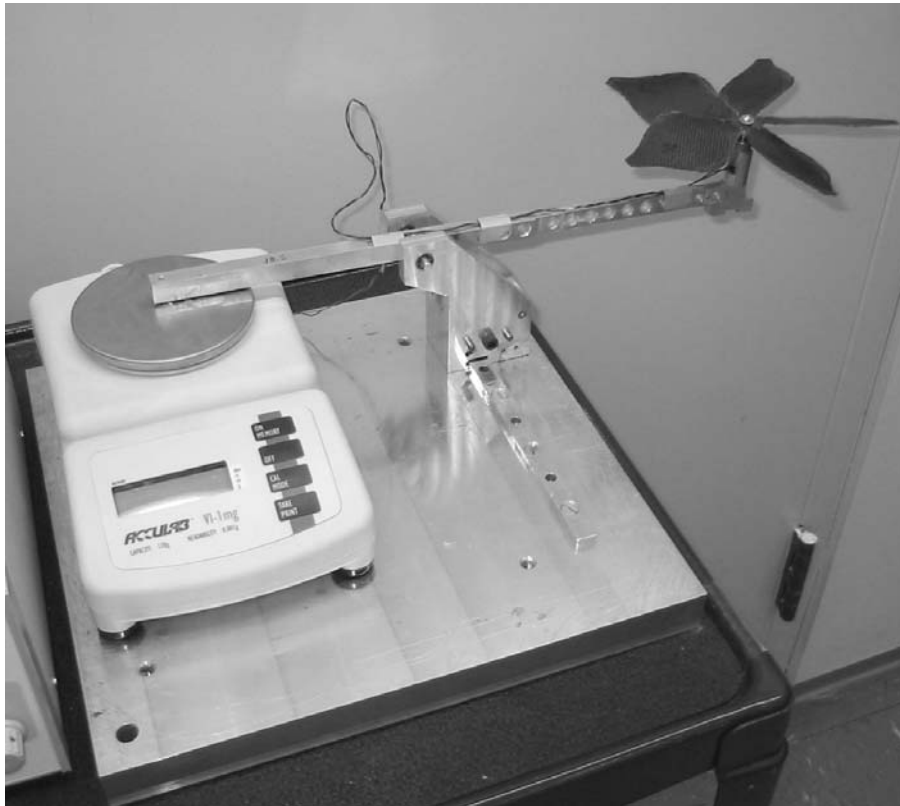
FIGURE 5.9 Large test fixture in thrust measurement configuration.
