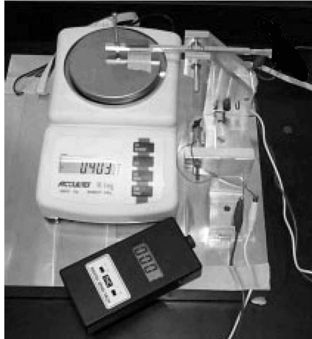
FIGURE 5.8 Motor testing experimental configuration.
