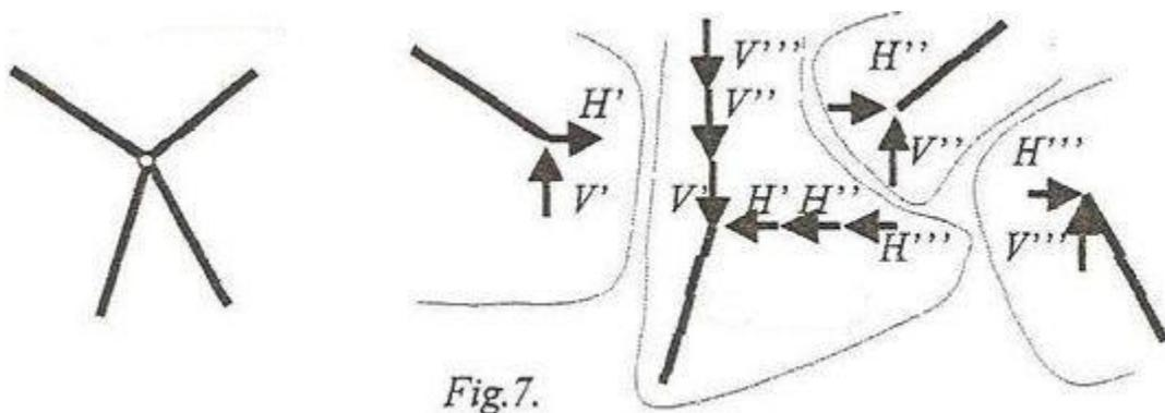
*The resulted scheme is the **free body diagram** corresponding to this method.*
