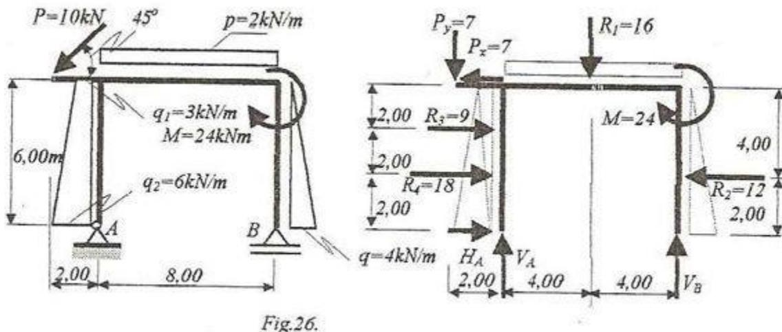
**Solution. Step 1.** The body is statically determined and stable because it has a hinge and a simple support, and the direction of the simple support doesn't pass through the hinge.
