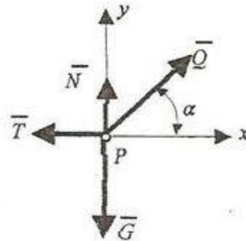
**Solution.** The particle has only one constraint with friction (the horizontal rough surface) because the string is not a constraint. Having one single constraint the particle has one degree of freedom, so it has one possibility of motion to slide on the horizontal plane. Because the force  $Q$  the particle has the tendency to move on the right sense.
