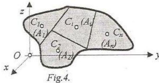
We shall consider the plate divided into simple plates for which we know the areas and the positions of the centroids. The  $x_C$  coordinate of the centroid of the whole plate is calculated:
