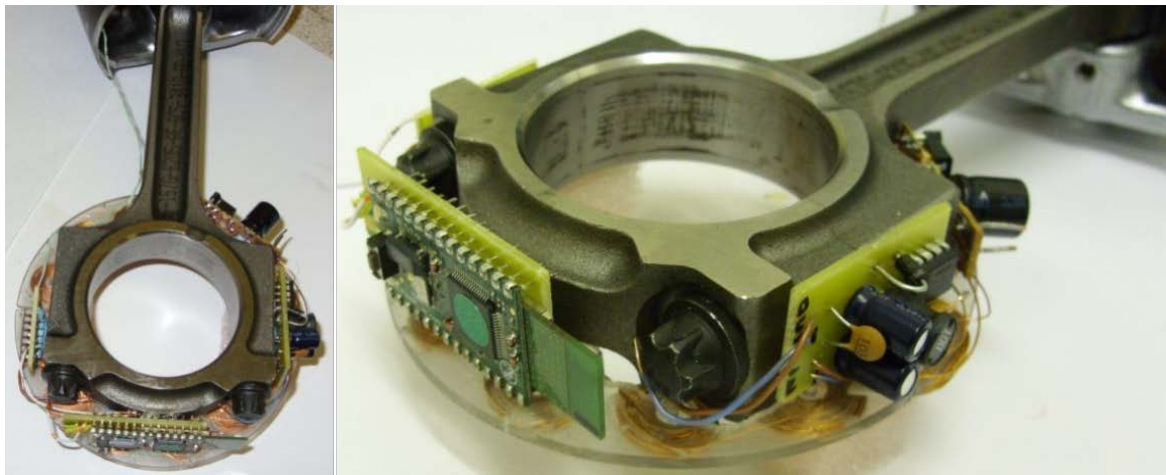
Figure 4. Coil ring and magnet disc a) individually b) adjacent. Telemetry electronics positioned on big end
