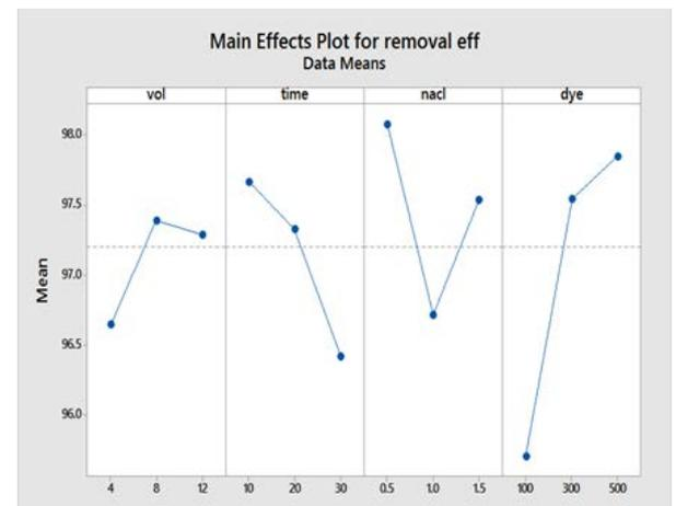
**Figure 6. Main effects plot for Removal Efficiency of Brilliant Green Dye**
