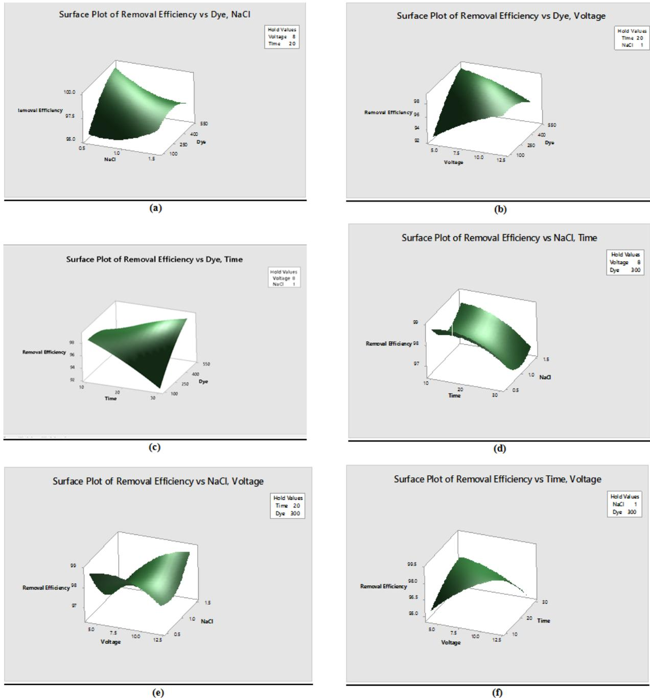
**Figure 7.** 3-D plots for Removal Efficiency of Brilliant Green Dye as a function of (a) initial dye concentration and NaCl conc. (b) initial dye concentration and voltage (c) initial dye concentration and time (d) NaCl conc. and time (e) NaCl conc. and voltage (f) time and voltage
