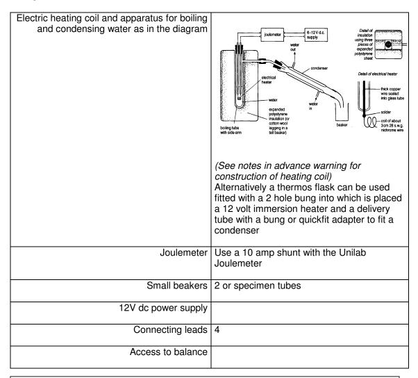
The experiment should be started using hot water as it takes a long time for the 12V immersion heater to boil the water from cold
