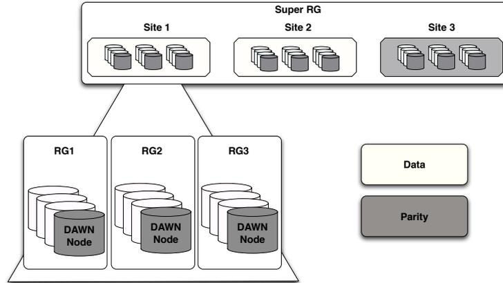
Figure 4: A visualization of our inter-device and inter-site reliability schemes for DAWN. Devices coordinate with each other to form reliability groups for ECC (or replica) management within sites. Entire sites may be similarly aggregated to form a super reliability group to withstand entire site failures.
