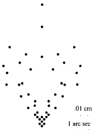
Figure 14.10 Spot diagrams for a Dall–Kirkham telescope.
