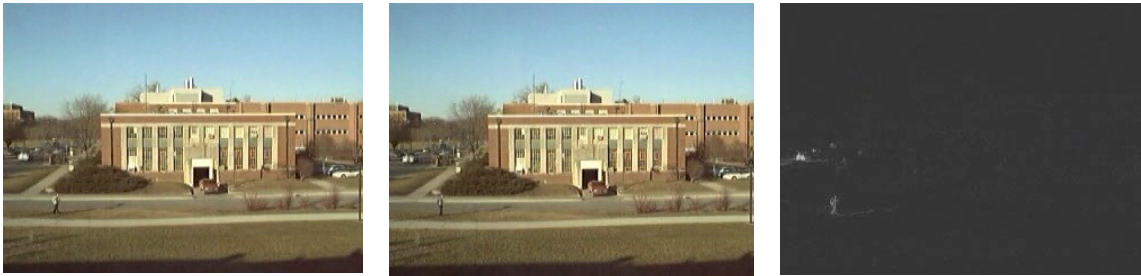
Figure 4.7a: Live image Frame1 Figure 4.7b: Live image Frame2 Figure 4.7c: Frame Difference
