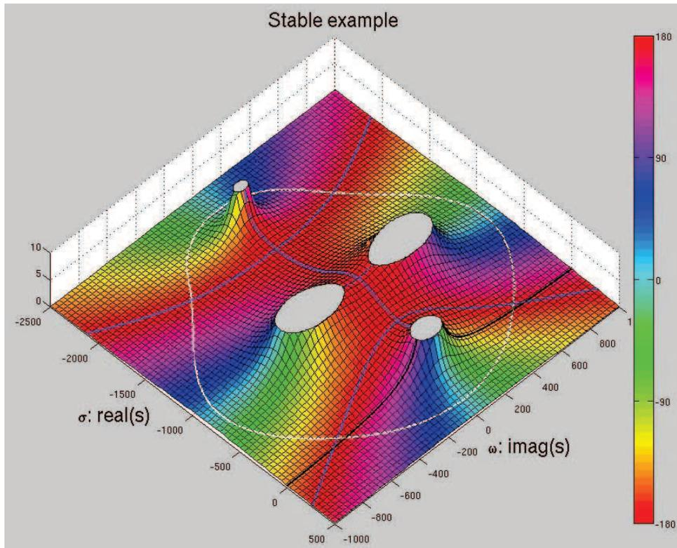
Figure 5: A stable four pole open loop gain function
