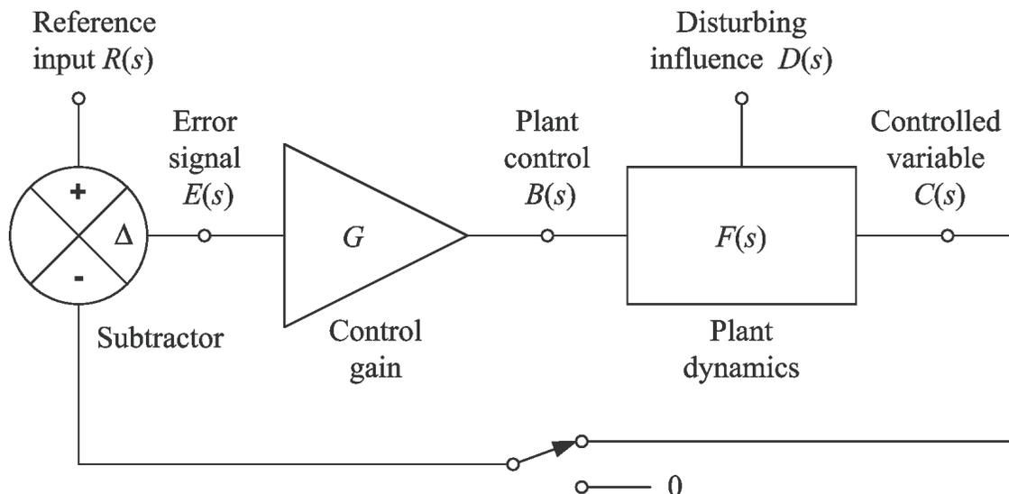
Figure 1: Model of a SISO control loop
