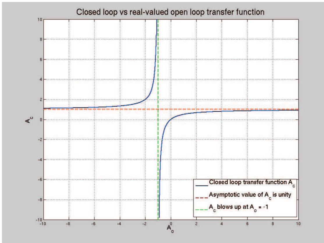
Figure 3: Four quadrant plot of closed and open loop gains
