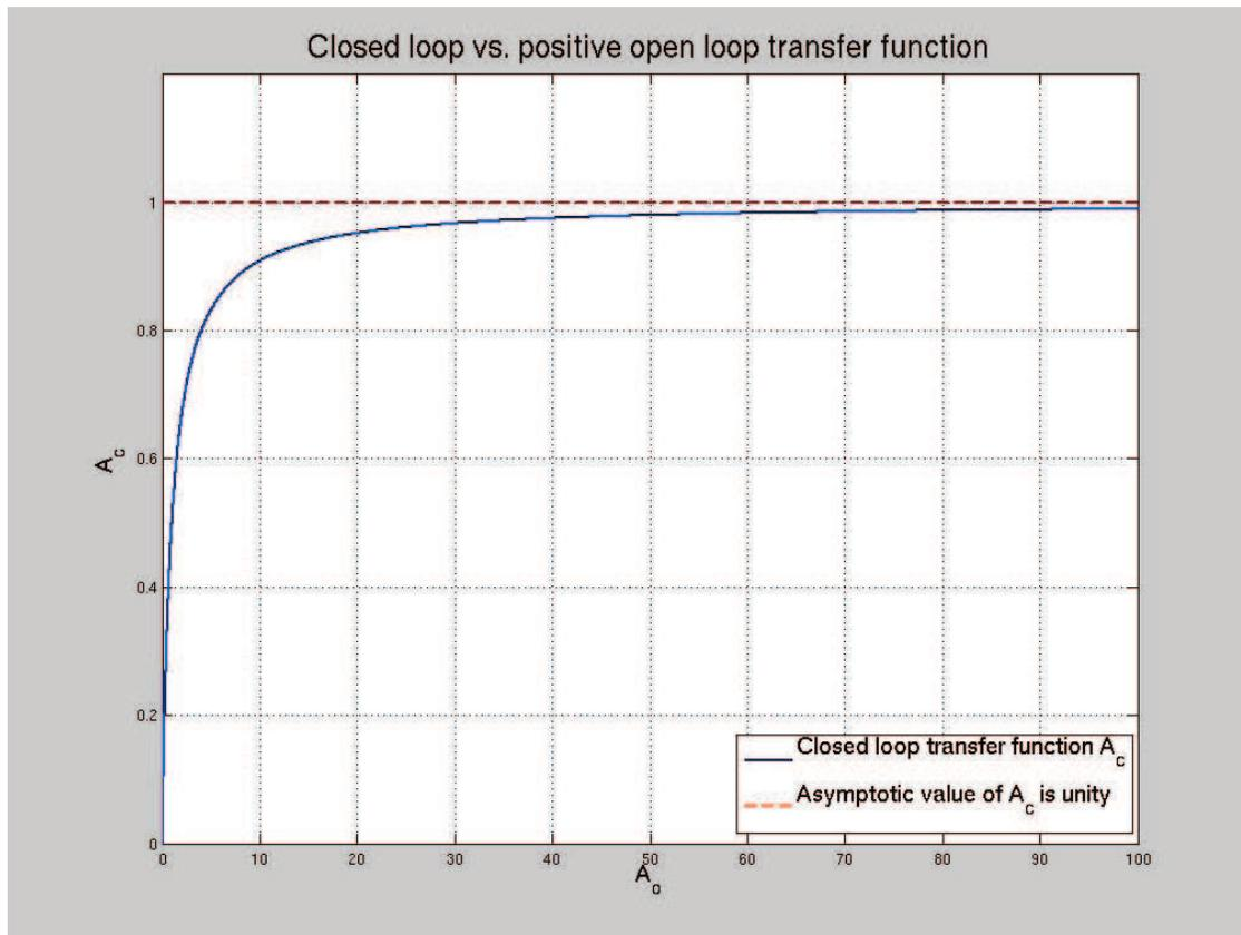
Figure 2: Closed and open loop gains vs reference input
