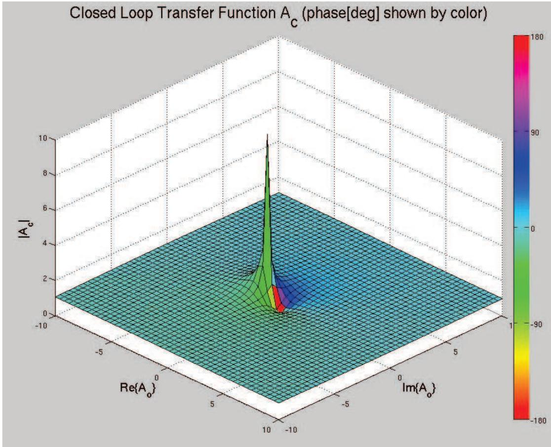
Figure 4: Complex closed loop gain vs. complex open loop gain
