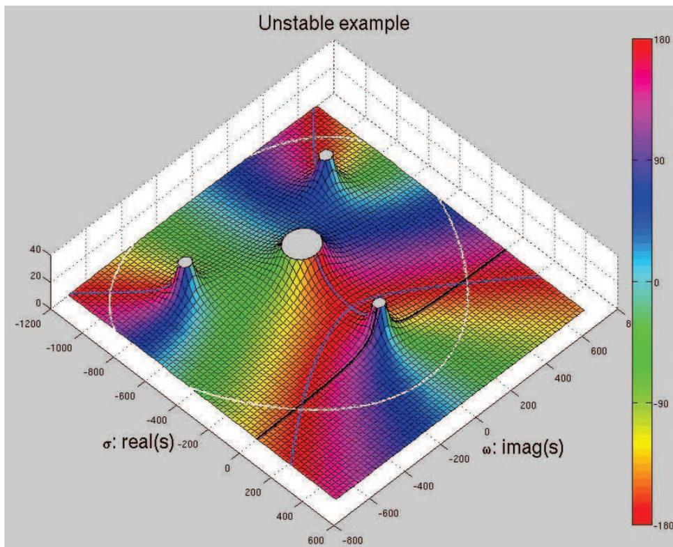
Figure 6: An unstable four pole open loop gain function
