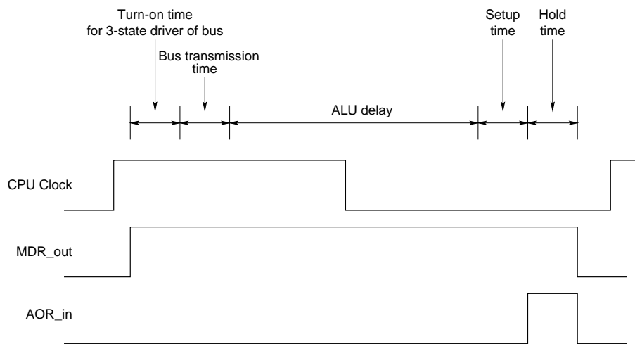
Figure 10.33: Control Signal Timing for Interpreting an ALU Microinstruction
