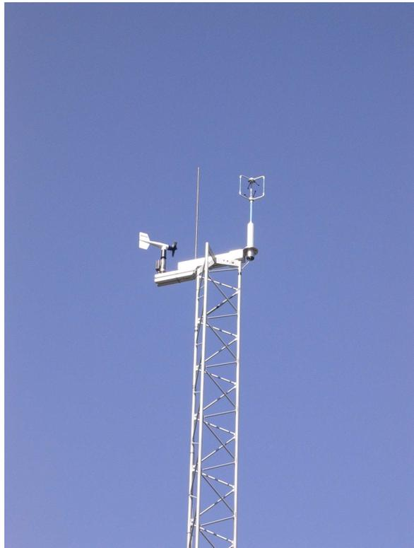
**Figure 1.8** The mast on which the anemometer is installed.
