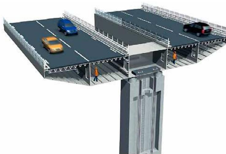
**Figure 1.2** Section of the bridge deck.
