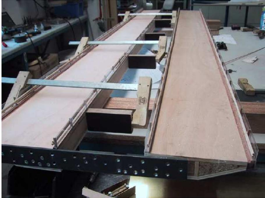
**Figure 2.16** Model of the cross section during modification for the tests on each box separately.
