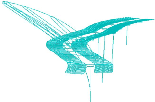
**Figure 4.79** Deformed configuration due to static equivalent forces.
