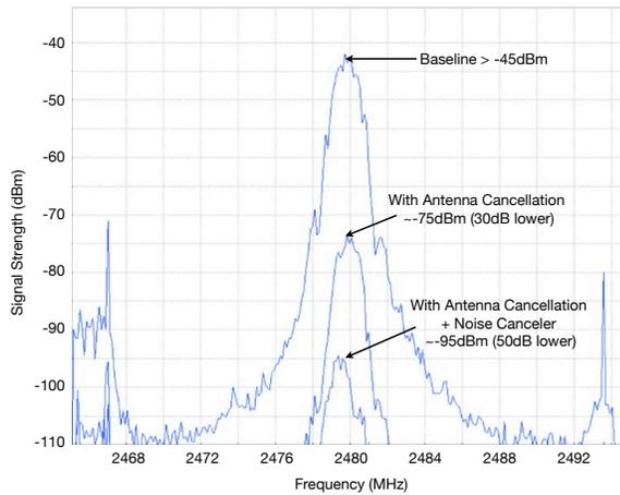
**Figure 7: Spectrum snapshots showing the effect of antenna cancellation and a combination of antenna and RF interference cancellation. A combination of the two techniques can give a  $\sim 50\text{dB}$  reduction in self-interference.**
