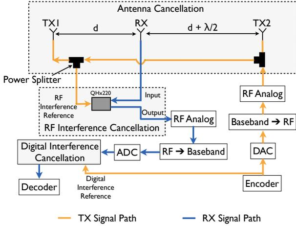
**Figure 2: Block diagram of a wireless full-duplex node. Colored blocks correspond to different techniques for self-interference cancellation. The power splitters introduce a 6dB reduction in signal, thus power from TX1 is 6dB lower compared to power from TX2, without the need for an additional attenuator.**
