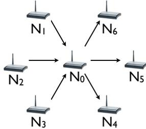
Figure 12: A star topology multihop network. Node  $N_0$  becomes a congested node. The network throughput in regular MAC operation is  $1/n$  for  $2n+1$  nodes.
