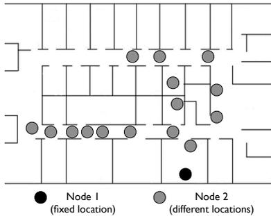
**Figure 8: Map of node locations for the experimental setup. Node 1 is always kept at a fixed location inside an office room and Node 2’s location is changed for each iteration to different locations within a building wing.**
