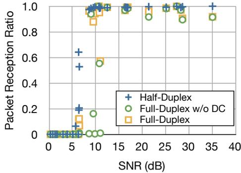
**Figure 10: Packet reception ratio vs SNR for different links. Full-Duplex achieves a similar SNR curve as half-duplex, but it shows lower PRR for high-SNR links.**
