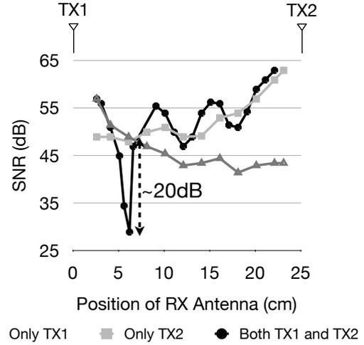
**Figure 5: Received SNR for different receive antenna placements. The received SNR is fairly monotonic with distance when any one transmit antenna is active. With both transmit antennas active, there is a sharp reduction in receive power at the null point.**
