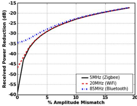
**Figure 4: Variation of received power at the null position with amplitude mismatch. An amplitude mismatch of 10%, corresponding to 1dB variation, can restrict the receive power reduction to  $\sim 20$ dB**
