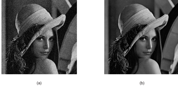
Figure 3: Pan threshold: (a) Direct thresholding ( \text{SNR} = 18.273 \text{ dB} ) (b) ANC following inverse thresholding ( \text{SNR} = 24.102 \text{ dB} )
