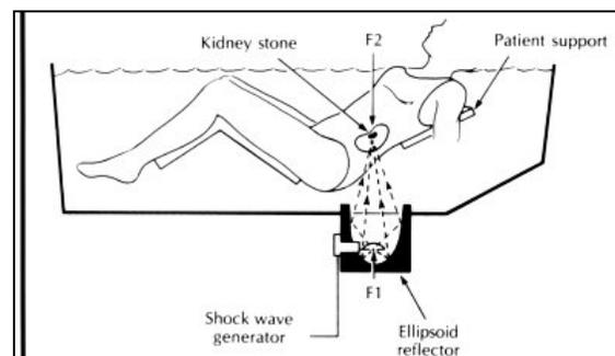
*In a lithotripter, sound is focused using an ancient property of ellipsoids*
