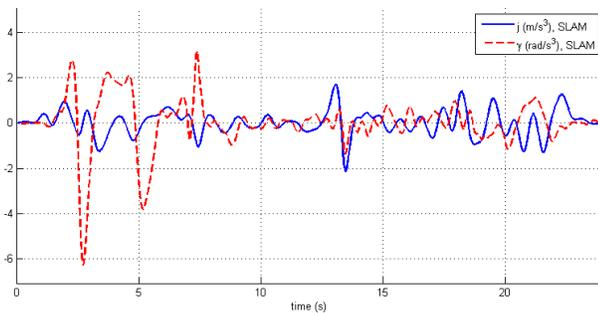
Figure 3.11: Jerks along the example robot trajectory
