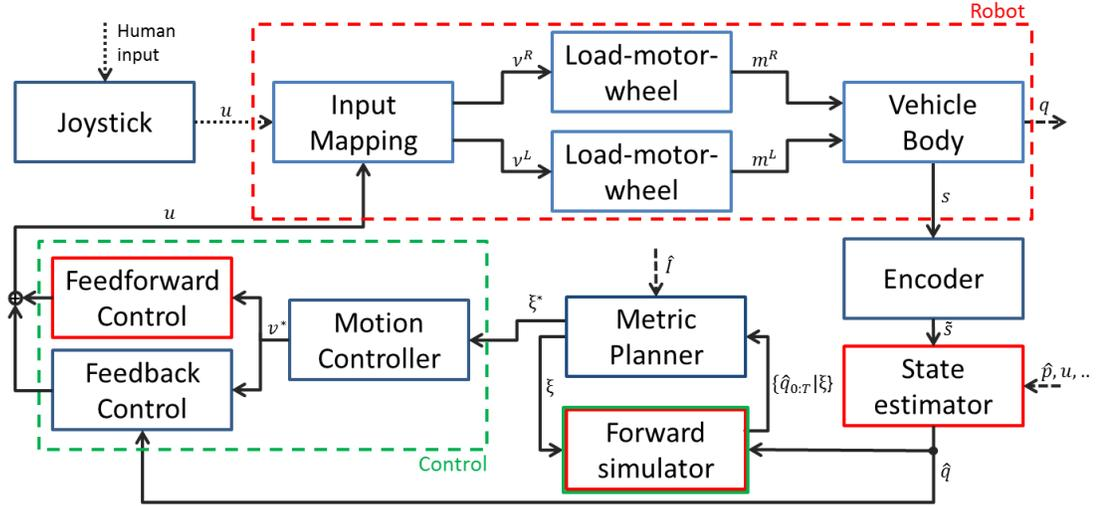
Figure A.1: Vulcan system diagram.
