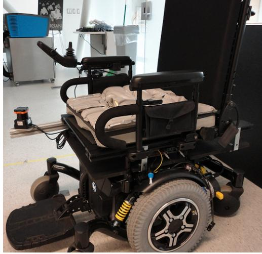
Figure 3.7: Differentially driven wheelchair robot.
