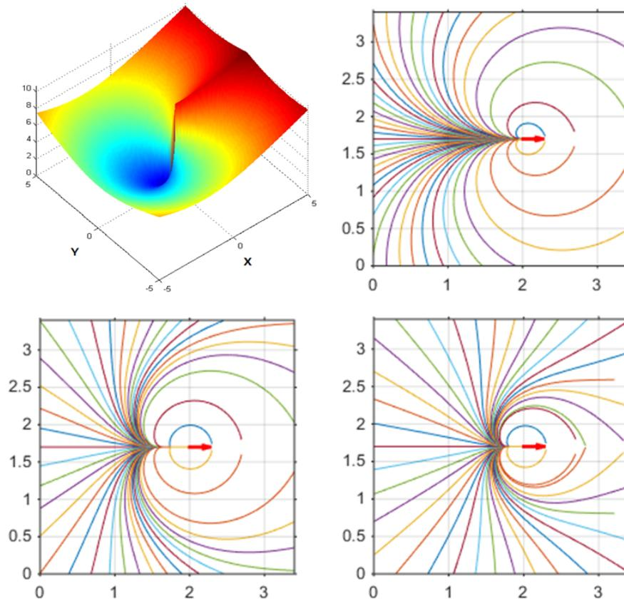
Figure 4.2: Visualization of a non-holonomic distance function, and example paths tracing user-specified vector fields.
