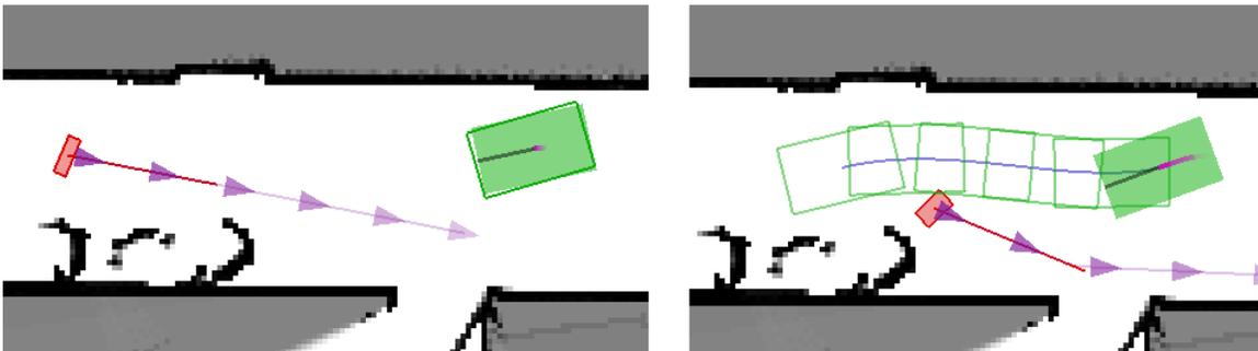
Figure 6.19: Snapshot of the policy and trajectory optimization that allows the robot to wait for a person to pass.
