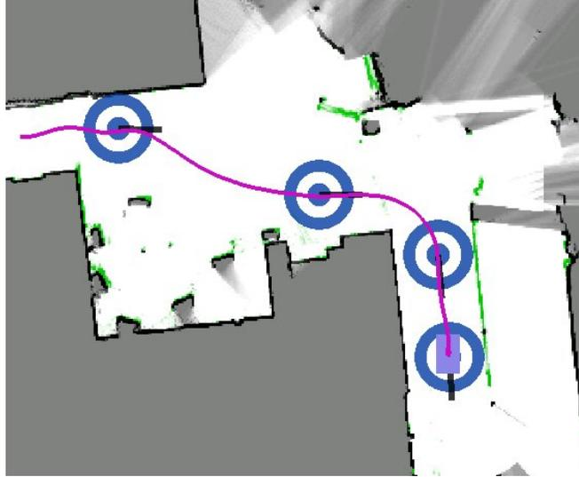
Figure 3.8: Example robot trajectory via static motion targets.
