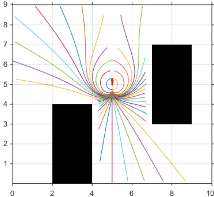
Figure 4.3: Estimating the domain of attraction in structured environments.
