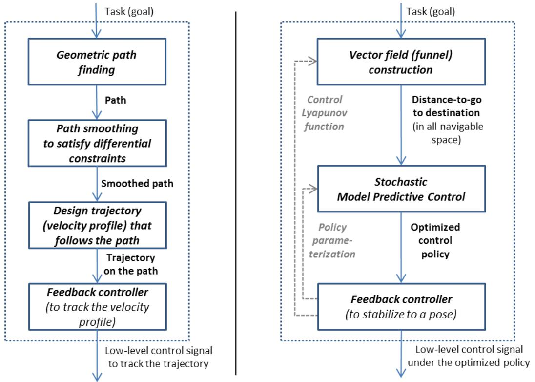
Figure 1.1: Motion planning and control architectures: Traditional vs. Ours.
