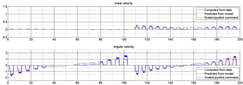
Figure A.3: The model prediction vs. measurements at low velocities with step inputs.
