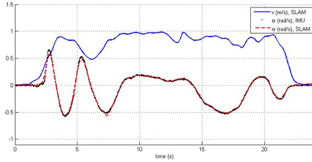
Figure 3.9: Velocities along the example robot trajectory
