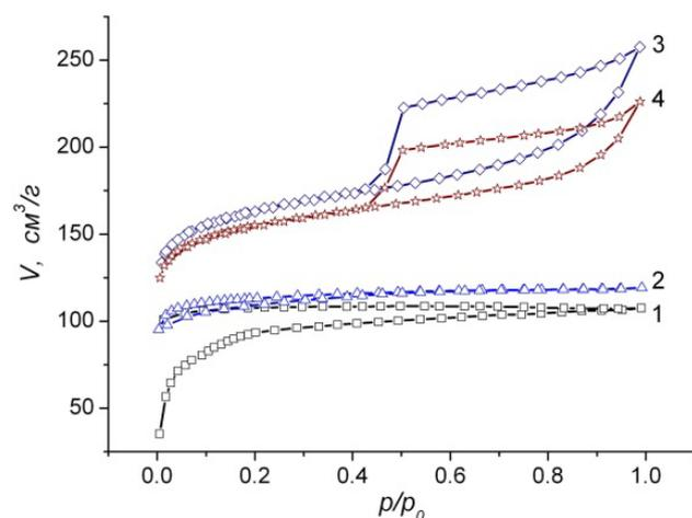
**Figure 1.** The sorption isotherms of initial PCM (1) and modified ones at temperatures of  $300$  (2),  $400$  (3), and  $500^{\circ}\text{C}$  (4)
