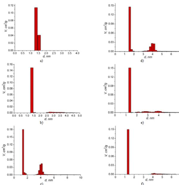
**Figure 2.** Pore size distribution of PCM at different modes of modification: a) initial sample; b)  $T_{mod} = 300^{\circ}\text{C}$ ,  $t_{mod} = 2,5$  h; c)  $T_{mod} = 400^{\circ}\text{C}$ ,  $t_{mod} = 2,5$  h; d)  $T_{mod} = 500^{\circ}\text{C}$ ,  $t_{mod} = 3$  h; e)  $T_{mod} = 600^{\circ}\text{C}$ ,  $t_{mod} = 0,25$  h; f)  $T_{mod} = 600^{\circ}\text{C}$ ,  $t_{mod} = 1$  h
