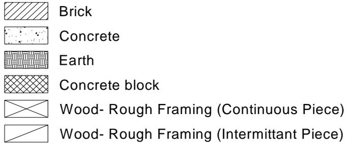
Figure 5. Examples of material symbols in section
