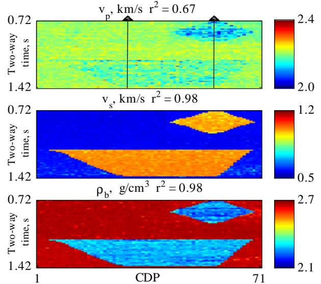
Figure 2. Cross-sections of the mean of inverted compressional-, shear-wave velocities, and bulk density for ten independent realizations obtained with the proposed inversion algorithm. Global correlation coefficients ( $r^2$ ) are calculated with respect to the reference model of elastic properties.
