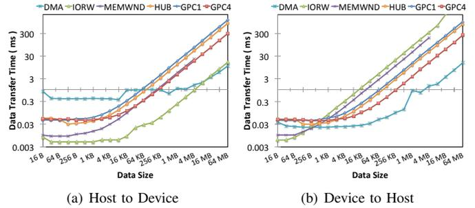
Fig. 10. The worst-case performance of the investigated data transfer methods using a real-time task under high CPU load.
