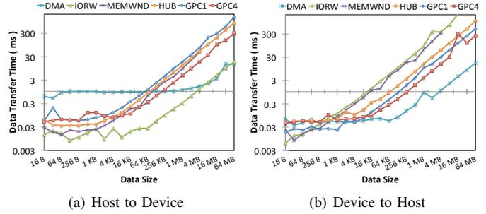
Fig. 14. Worst-case performance of each data transfer method with a real-time task under high memory pressure.
