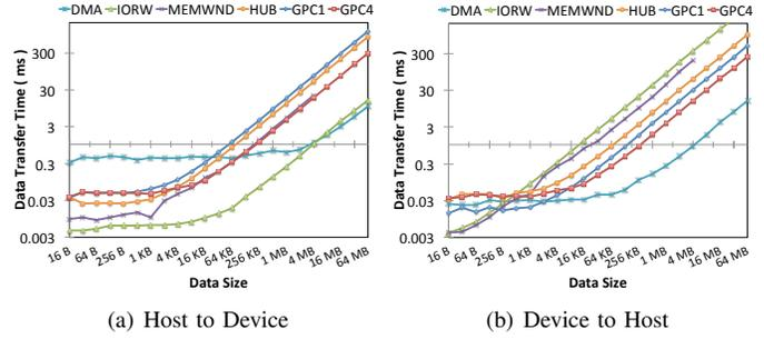
Fig. 13. Average performance of each data transfer method with a real-time task under high memory pressure.
