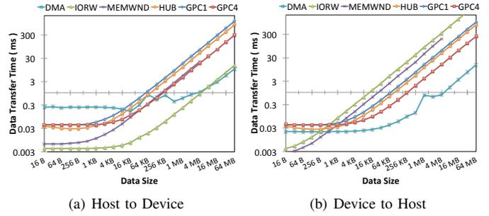
Fig. 9. The average performance of the investigated data transfer methods using a real-time task under high CPU load.
