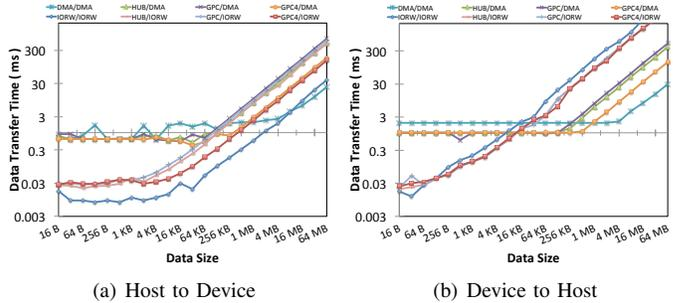
Fig. 18. The worst-case performance of the combined data transfer methods for concurrent real-time tasks.
