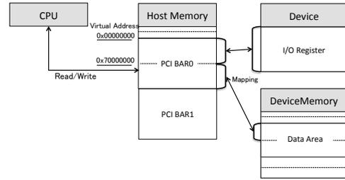
Fig. 6. Memory-window read and write.
