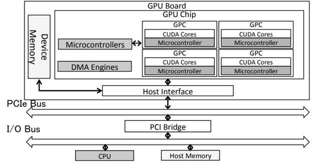
Fig. 2. Block diagram of the target system.
