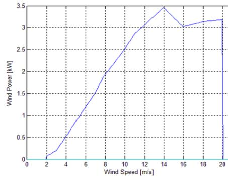
Figure 4. Power–wind speed curve of the wind generator
