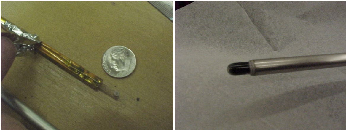
Figure 3.15: Left: Photo of a magnetic coil attached to a buffer amplifier prior to insertion in to a stainless steel probe shaft and glass cap. Right: Photo of magnetic fluctuation probe tip, showing glass cap (with graphite coating internally) attached to a 1/4" stainless steel shaft.
