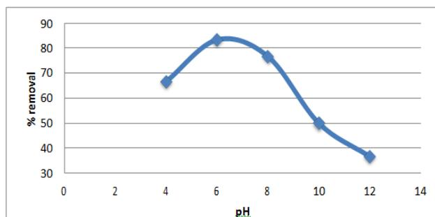
Figure 4. graph showing the effect of pH on Lead removal %
