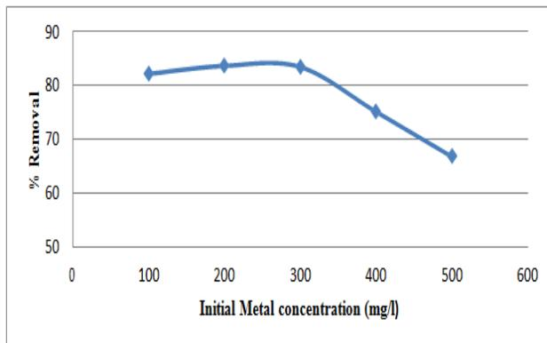
**Figure 5.** Effect of initial metal concentration on metal removal efficiency
