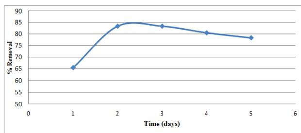
Figure 2. Effect of incubation time on lead removal efficiency
