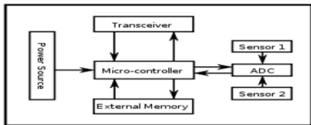
Fig.1 Block Diagram of a Mote
