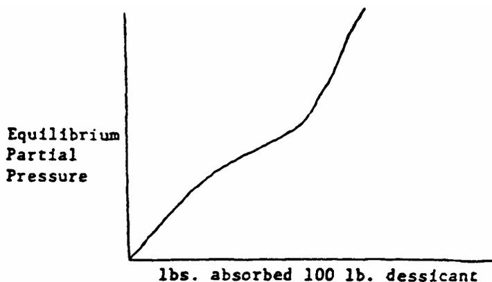
Figure 7.40: Adsorption Curve
