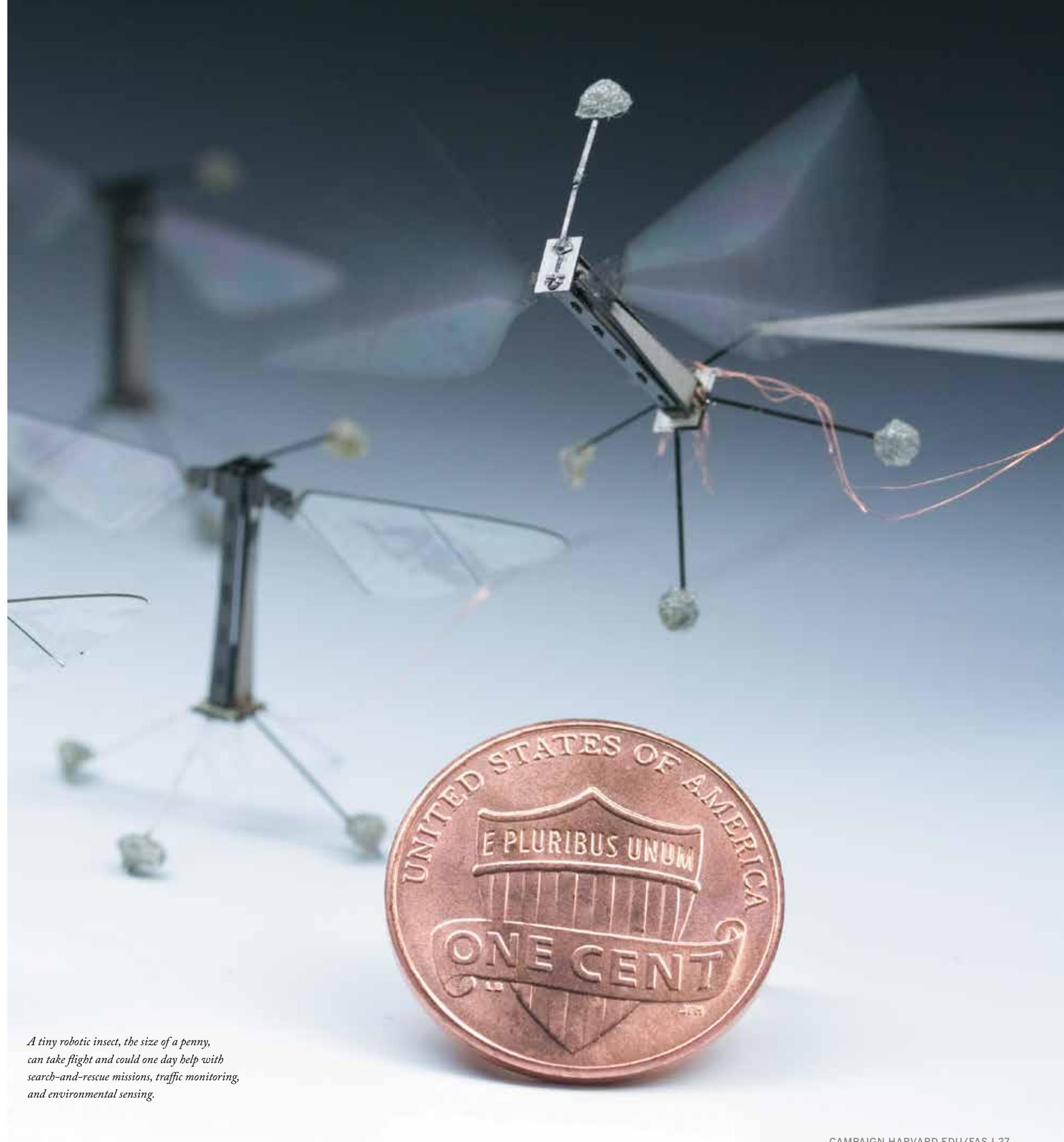
*A tiny robotic insect, the size of a penny, can take flight and could one day help with search-and-rescue missions, traffic monitoring, and environmental sensing.*
