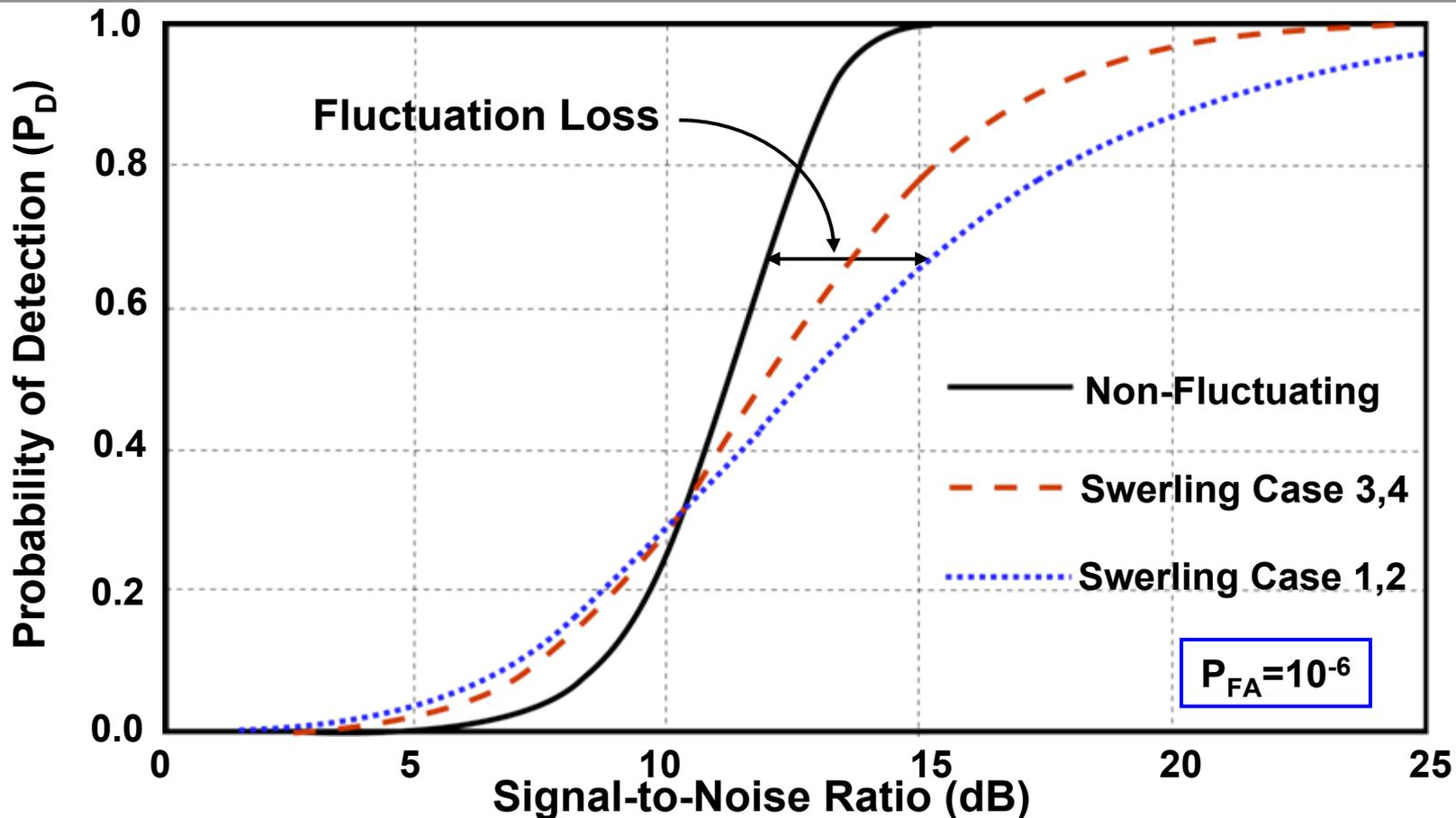
For high detection probabilities, more signal-to-noise is required for fluctuating targets.
