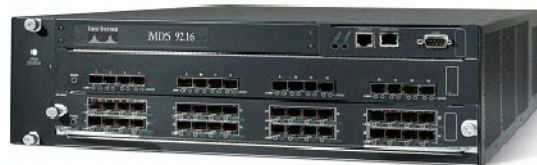
Figure 6-3 MDS 9216A Multilayer Switch (IBM 2062-D1A) with 48 ports
