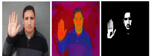
Fig. 7: a: face detection with harr cascade face, (b): HSV model, (c): Skin region Detection mask after thresholding and adequate morphological processing
