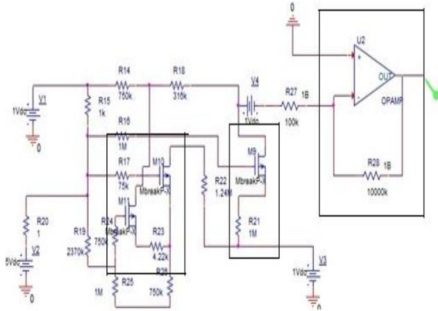
**FIGURE 2: Proposed Circuit of Gaussian membership function**
