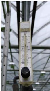
**Figure 16.** Model: H-03216-04: 65 mm variable area aluminum flow meter with valve and glass float for O<sub>2</sub>.
