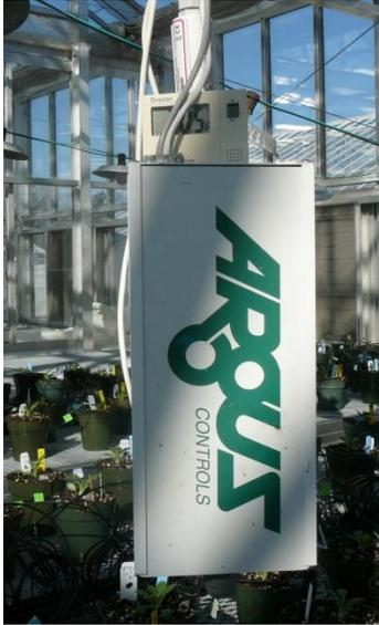
Figure 10. Aspirated box in a greenhouse. A fan draws air from the bottom of the box over the sensors.
