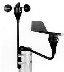
The data logger then uses known multiplier (or slope) and offset (or intercept) constants to calculate the actual wind speed.
