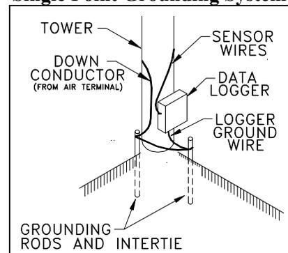
Their dimensions will determine the contact surface area with the soil, a key element for proper system grounding. A combination of the three can be used to enhance the contact area if they are all electrically connected.
