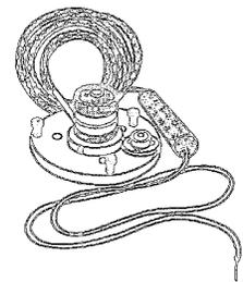
An output current is measured from both types by the data logger (or interface device), which uses a known multiplier and offset to calculate the global solar radiation. The current output is usually very small (microamps or less). Normally, the measuring instrument will have a “dropping” resistor and an amplifier that conditions the signal to obtain adequate output range.
