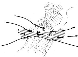
Features to be avoided include areas immediately upwind and downwind of higher terrain, the lee side of ridges, and excessively sloped terrain. In each of these situations, increased turbulence may occur.
