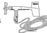
Although the two sensor types differ somewhat in their responsiveness to wind speed fluctuations, there is no clear advantage of one type over the other. In practice, the cup type is most commonly used for resource assessment.
