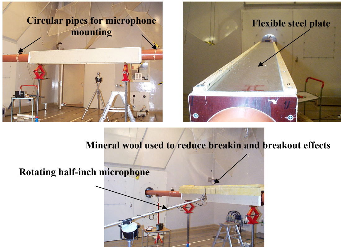
Figure 6: Measurement set-up in the reverberation room of MWL.
