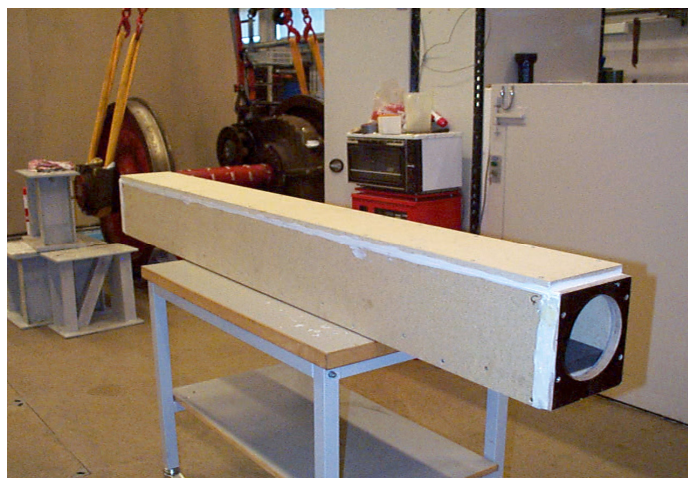
Figure 11: Rigid walled duct. The polyurethane foam is lined at the bottom.
