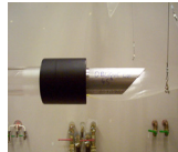
Figure 21: Modelling the opening reflection coefficient and impedance of oblique cuts.
