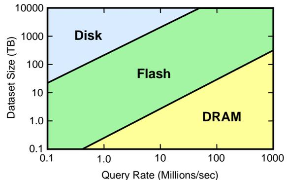
**Figure 2.** This figure (reproduced from Andersen et al. [1]) indicates which storage technology has the lowest total cost of ownership over 3 years, including server cost and energy usage, given the required dataset size and query rate for an application (assumes random access workloads).
