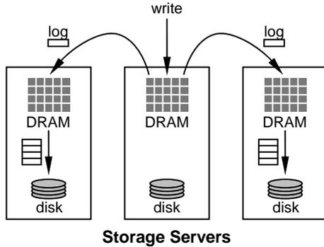
**Figure 3.** In the buffered logging approach to durability, a single copy of each object is stored in DRAM. When an object is modified, the changes are logged to 2 or more other servers. Initially the log entries are stored in the DRAM of the backup servers; they are transferred to disk asynchronously in batches in order to utilize the full disk bandwidth.
