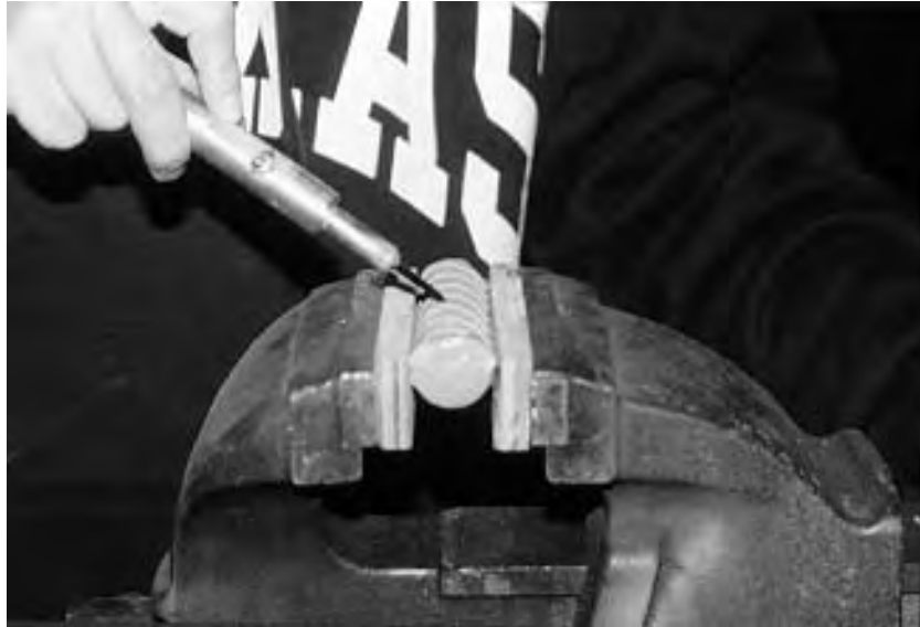
Figure 2.4 Adhesion testing of epoxy-coated bar specimen.
