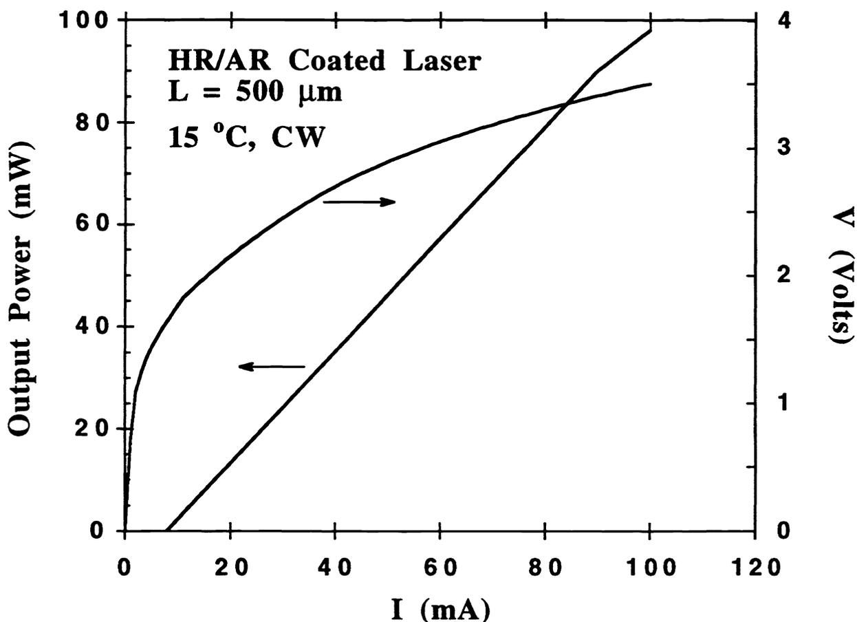
Fig. 5 A typical CW light-current characteristic for a  $500 \mu\text{m}$  long single QW ridge waveguide ( $4 \mu\text{m}$  wide) laser with high-reflective (85%) / anti-reflective (5%) coated facets.
