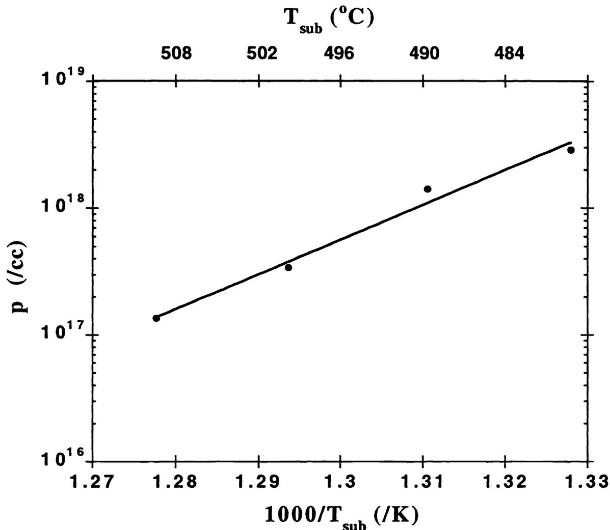
Fig. 2 The net hole concentration dependence on the substrate temperature for a fixed diethylzinc flow of 3 sccm and GaInP growth rate of 6.5 Å/s.
