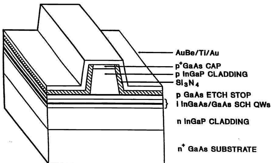
Fig. 3 A schematic of the self-aligned ridge-waveguide InGaAs/GaAs quantum well laser with lattice-matched GaInP cladding layers.
