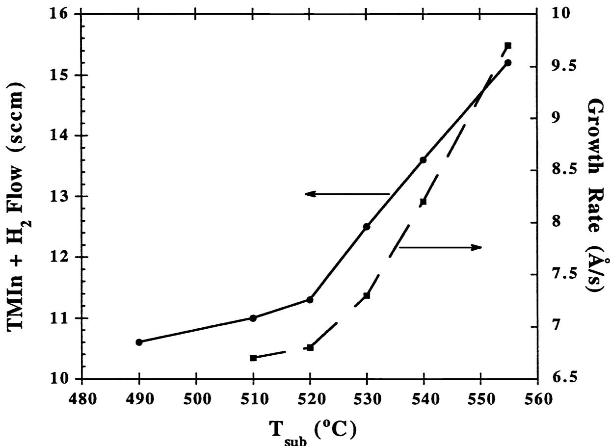
Fig. 1. The substrate temperature dependence of the  $\text{H}_2 + \text{TMIn}$  flow required to obtain lattice matching of GaInP on  $n^+$ -GaAs substrate and the  $\text{Ga}_{0.51}\text{In}_{0.49}\text{P}$  growth rate. The  $\text{H}_2 + \text{TEGa}$  flow and  $\text{PH}_3$  flow were kept constant at 12 sccm and 10 sccm, respectively.
