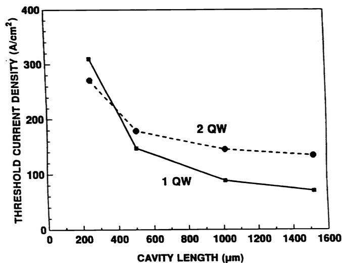
Fig. 4 The cavity length dependence of the threshold current densities,  $J_{\text{th}}$ , for broad-area lasers having a single and two quantum well
