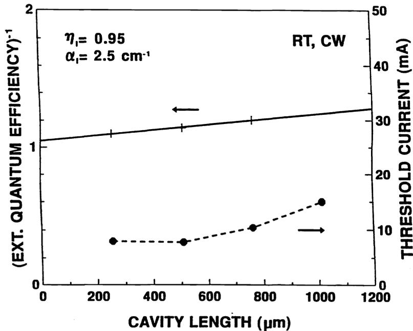
Fig. 6 The inverse external differential quantum efficiency and the threshold current versus the cavity length for single QW ridge waveguide lasers. The extrapolated internal quantum efficiency is 95% and the internal waveguide loss is  $2.5 \text{ cm}^{-1}$ .
