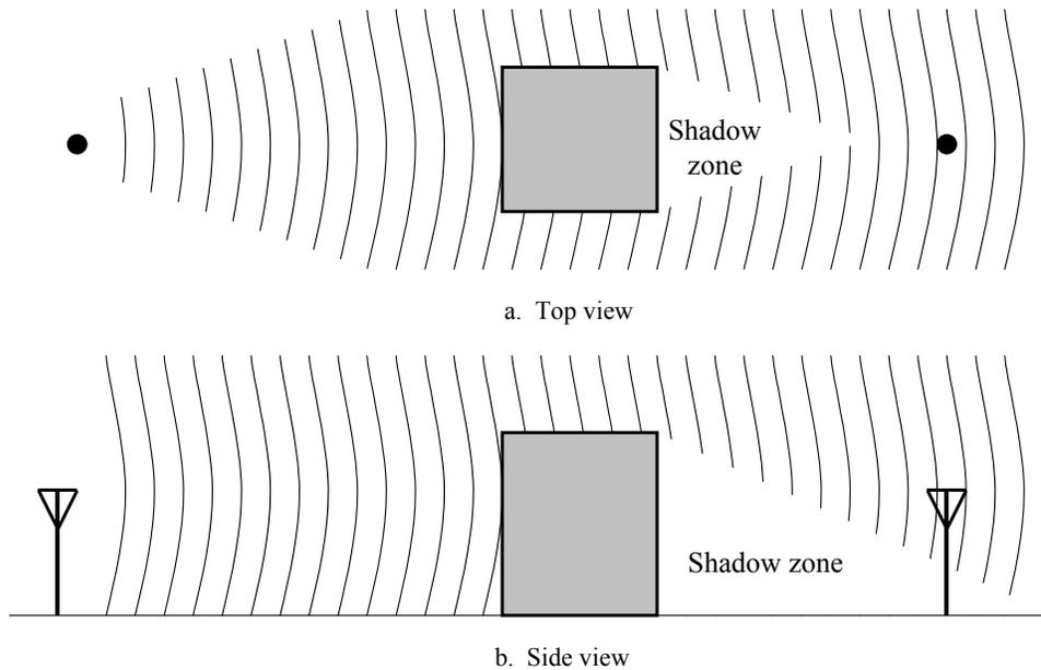
**Figure 1-13. Diffraction of a wave around a building**
