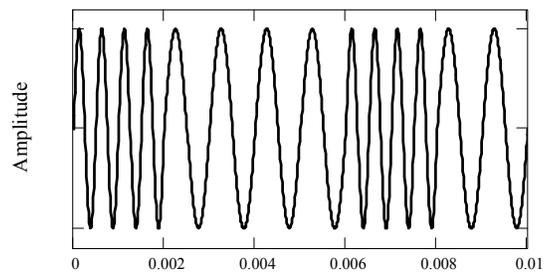
b. Frequency modulated digital signal
