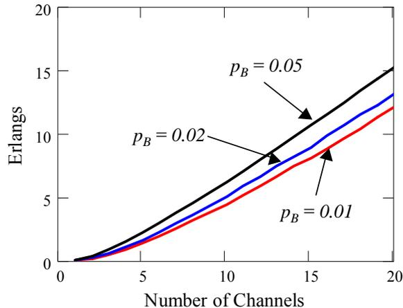
**Figure 7-8. Graph of the Erlang C formula showing the benefit of statistically multiplexing channels to support randomly arriving traffic<sup>11</sup>**
