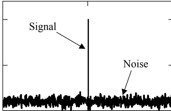
**Figure 1-21. Signal and noise in the frequency domain**
