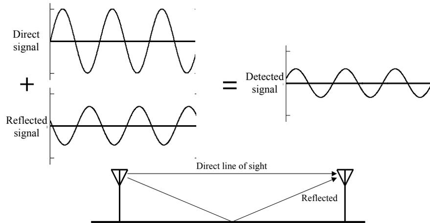
**Figure 1-15. Multipath interference**
