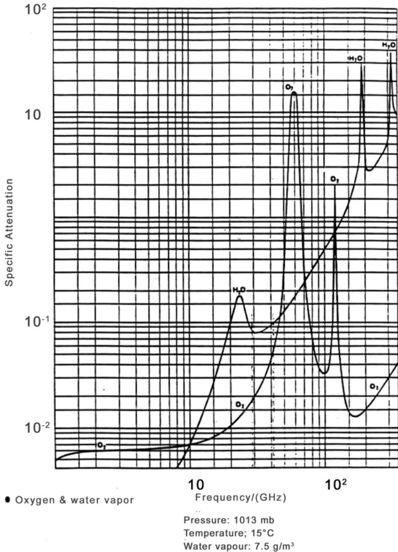
**Figure 1-22. EM signal absorption by atmospheric gases**
