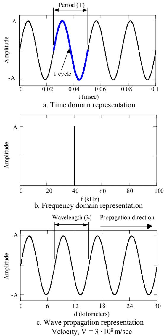
**Figure 1-1. Representations of a 40kHz sine wave**
