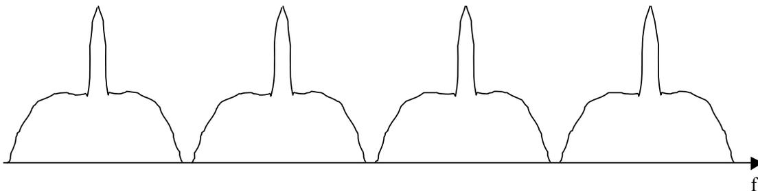
**Figure 1-10. Example of using different carrier frequencies to multiplex multiple signals on the same media**
