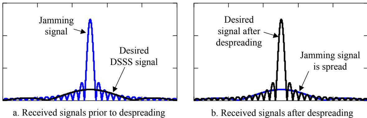
**Figure 7-5. Anti-jam characteristics of DSSS**
