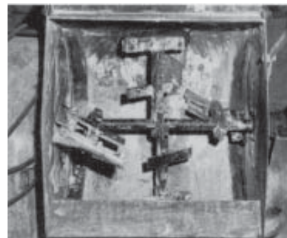
A paddle mixer is used for castables.
