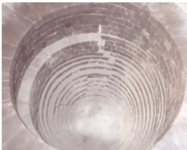
Photo shows AOD vessel with NARMAG® FG and SUPER NARMAG® 142 zoned by brand and thickness for optimal performance.
