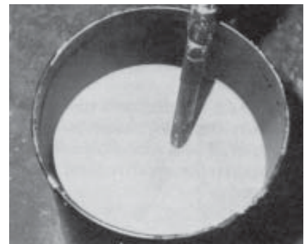
This contains too much water for vibration.
