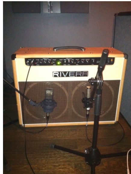
IMAGE 6a, 6b. MICROPHONE CONFIGURATION FOR ELECTRIC GUITAR: Jeff set up his guitar pedals as desired and plugged into the Rivera Amplifier. The Amplifier was then miked with Royer 121 Ribbon mike, an SM57, and a DI Box.
