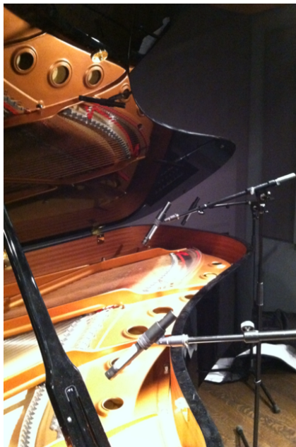
IMAGE 3a, 3b. MICROPHONE CONFIGURATION FOR TRACKING GRAND PIANO: In the final mixes, 2 DPA 4011 microphones were directed at a 30-degree angle at the mid and high strings of the piano as recommended by DPA's website.
