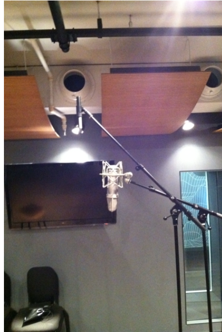
IMAGE 3a, 3b. MICROPHONE CONFIGURATION FOR TRACKING GRAND PIANO: In the final mixes, 2 DPA 4011 microphones were directed at a 30-degree angle at the mid and high strings of the piano as recommended by DPA's website.
