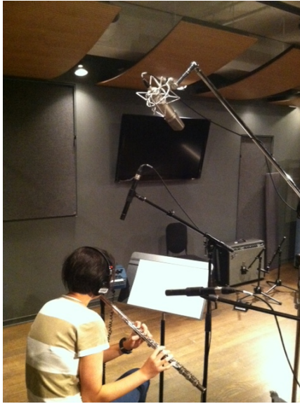
IMAGE 5a, 5b. MICROPHONE CONFIGURATION FOR FLUTE & UKULELE: The flute and ukulele were both miked overhead with a Neumann U87 and then close miked with 2 spaced DPA 4011 microphones.
