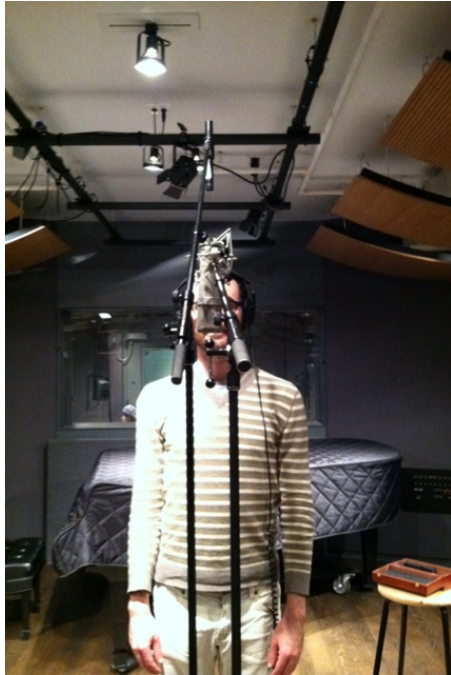
IMAGE 3a, 3b. MICROPHONE CONFIGURATION FOR TRACKING GRAND PIANO: In the final mixes, 2 DPA 4011 microphones were directed at a 30-degree angle at the mid and high strings of the piano as recommended by DPA's website.
