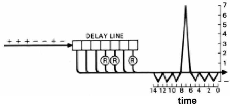
Correlation process may be performed in analog or digital domain. A disadvantage of this approach is that the data acquisition system (A/D converter) must operate at the full system bandwidth (e.g., 1 GHz in our example).
