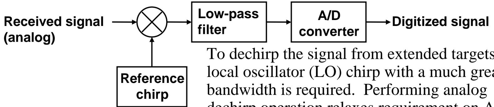
To dechirp the signal from extended targets, a local oscillator (LO) chirp with a much greater bandwidth is required. Performing analog dechirp operation relaxes requirement on A/D converter.
