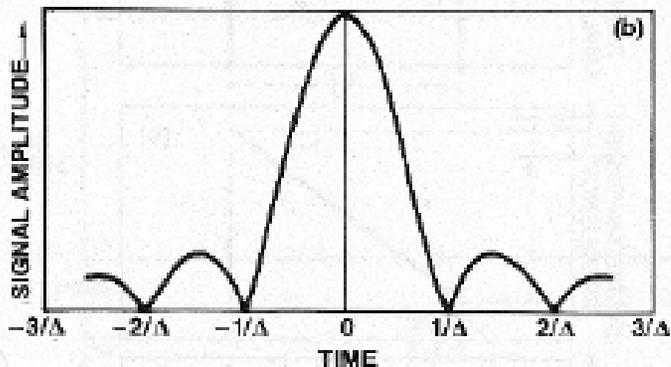
**Peak sidelobe level can be controlled by introducing a weighting function -- however this has side effects.**
