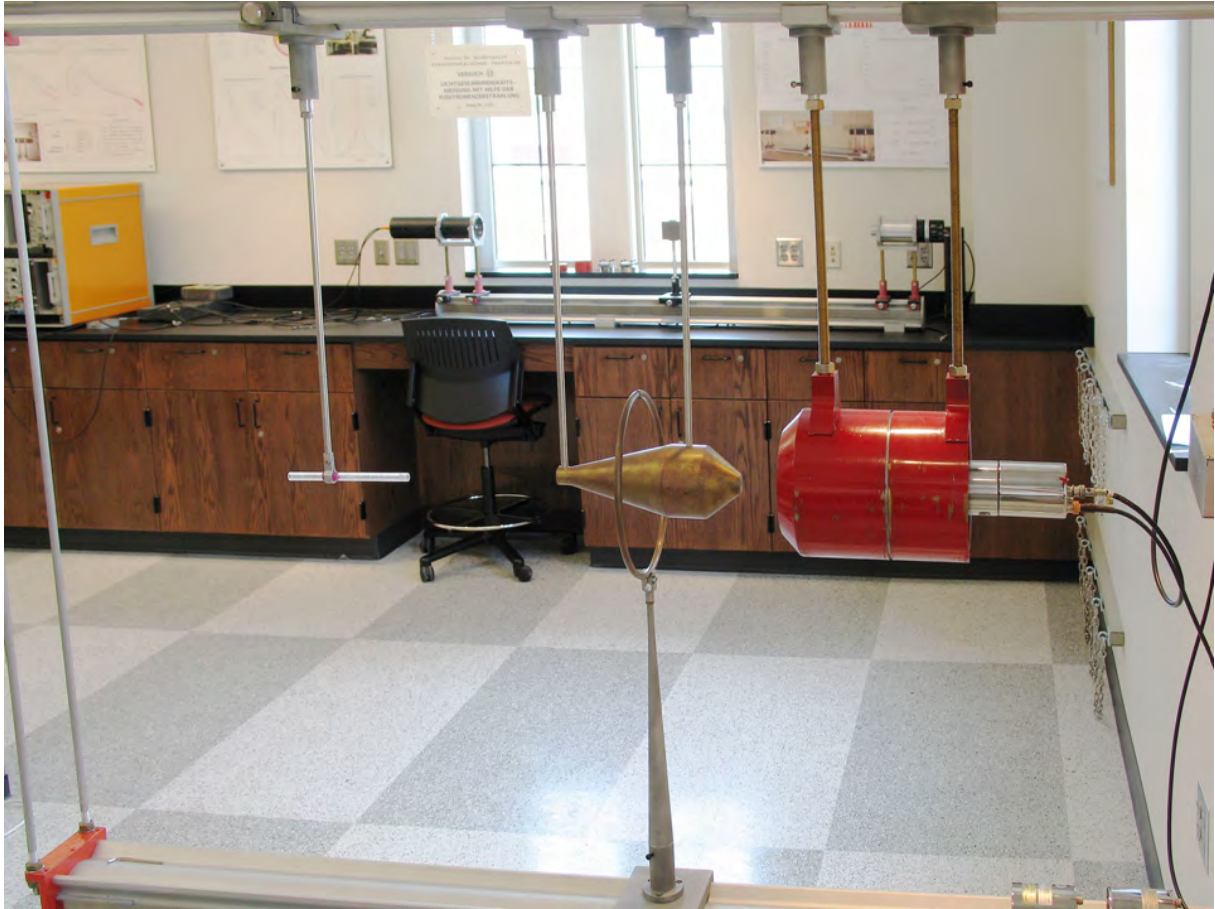
Figure 47: Other view of the Compton experiment setup with central parts: source, ring-sample, shadow-bar, detector
