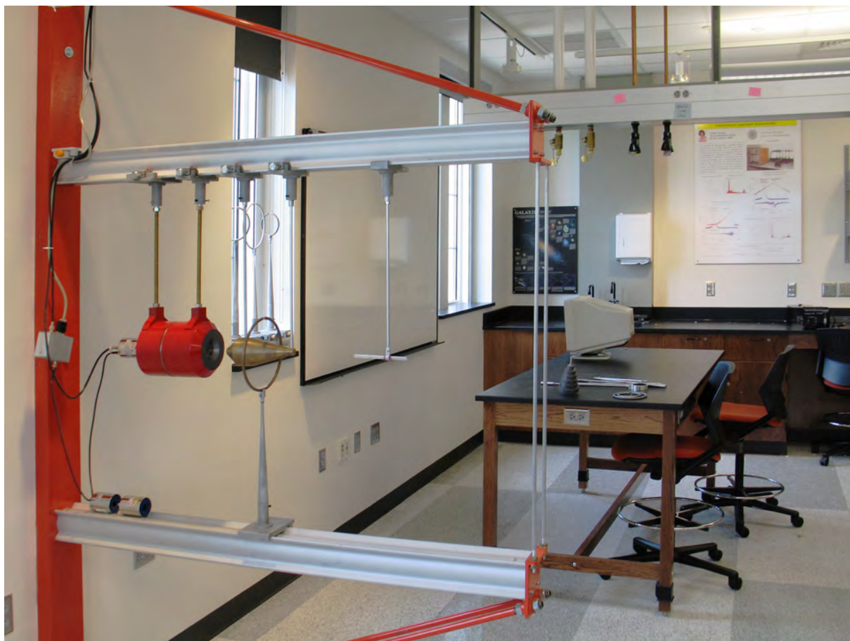
Figure 46: Set-up of the the Compton experiment with ring geometry for cross section determination. Note the considerable distances for all structural elements which contribute to background
