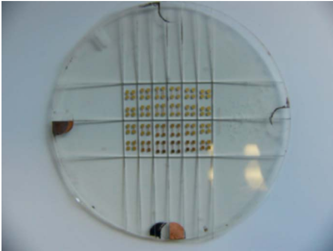
Fig. 2. Fabricated micro-inductors on a pyrex glass wafer by MEMS technique.
