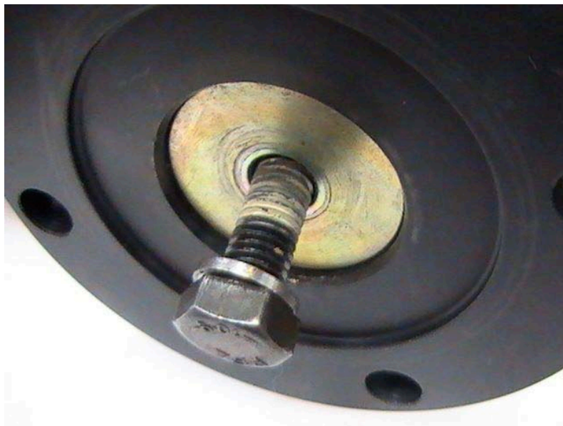
Figure 2-41: A setscrew which has been locked in place with a compound similar to Loctite, then forcibly unscrewed. The remains of the locking compound can be seen as the yellowish substance on the threads of the setscrew. In this particular application, the locking compound also served to seal the thread to prevent oil from inside the housing from leaking out along the spiral of the thread.
