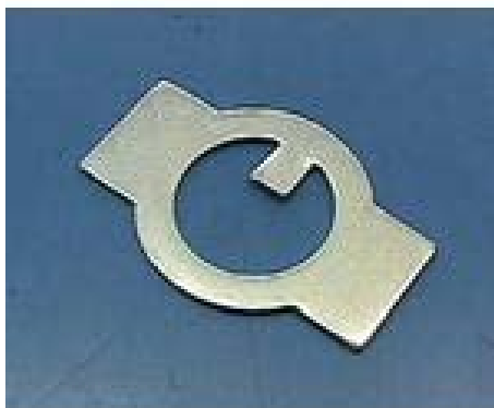
Figure 2-37: Examples of LOCK TABS or TAB WASHERS or LOCK WASHERS . These washers are intended to fit onto a threaded length of a bolt or shaft in which a longitudinal slot called a KEYWAY has been machined. The central tab prevents rotation of the washer on the shaft and one of the outer tabs is bent up to lock the nut in position. See Fig 2-38. http://www.smallparts.com.au/store and http://www.minibearings.com.au/store/categories/washers
