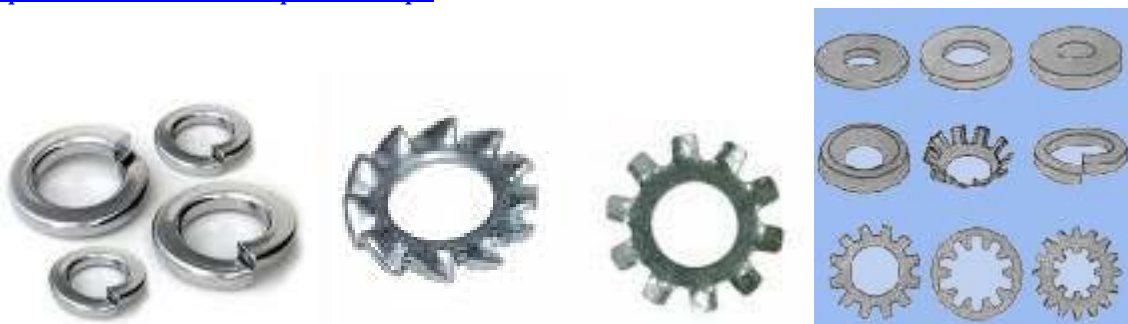
Figure 2-35: Left: SPRING WASHERS or SPLIT WASHERS which work by allowing tightening to proceed normally but prevent loosening by digging in the sharp edges of the split if the nut tends to loosen. The washers shown are for right-hand threads.
