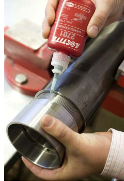
Figure 2-40: Showing Loctite products being applied to the threaded section of a shouldered or stepped bolt in a crankcase assembly and to a sleeve being inserted into a cylindrical component. It is only necessary to apply a few drops of the Loctite compound, which hardens and secures in the absence of oxygen.
