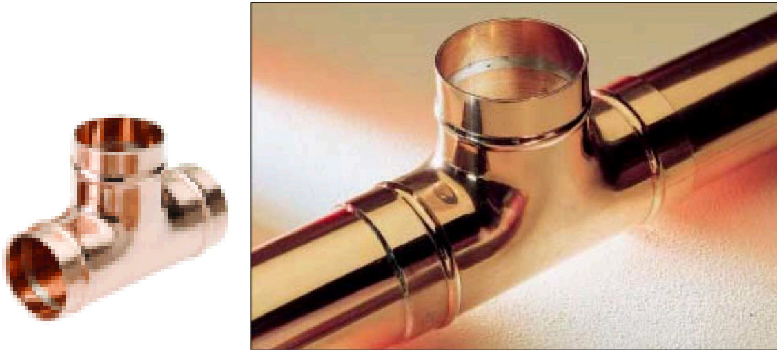
Figure 2-53: An example of a proprietary soldered fitting known as a Yorkshire fitting. Copper pipes have already been soldered into two of the openings of the T-piece on the right. A thin ring of solder is visible in the upright opening. When a clean and flux-covered copper pipe is inserted into the upright opening and the T-piece heated, the solder melts, spreads over the whole contact area, and forms a strong pressure-tight joint. http://www.pegler.com/EN/Products/Yorkshire/General
