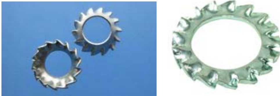
Left: Conical serrated lock washers, used with countersunk-head screws.
