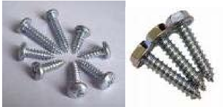
Figure 2-20: Self tapping screws, round head and hexagonal head. These screws are screwed into pre-drilled holes in sheet metal, plastic or timber and cut their own coarse thread.
