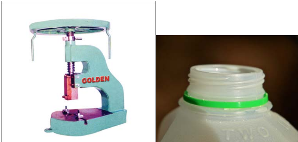
Figure 2-14: An example of a multi-start thread can be found on some hand operated BENCH FLY PRESSES (left). The large FLYWHEEL on top of the press is rotated by hand and, as it rotates, raises or lowers the press tool (the red portion of the press) by means of the MULTI-START THREAD . The kinetic energy stored in the rotating flywheel is utilised to carry out operations such as light riveting or staking. http://product-image.tradeindia.com
