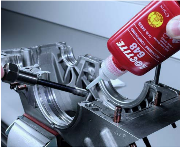
Figure 2-40: Showing Loctite products being applied to the threaded section of a shouldered or stepped bolt in a crankcase assembly and to a sleeve being inserted into a cylindrical component. It is only necessary to apply a few drops of the Loctite compound, which hardens and secures in the absence of oxygen.
