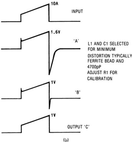
**FIG. 3.15.1** (a) Low-cost oscilloscope current probe for high-frequency unidirectional current pulse measurement. (b) Input current waveforms and output voltage analogues of oscilloscope current probe: Top, primary input current; A, voltage waveform, secondary; B, voltage waveform after ferritification; C, voltage waveform after shaping
