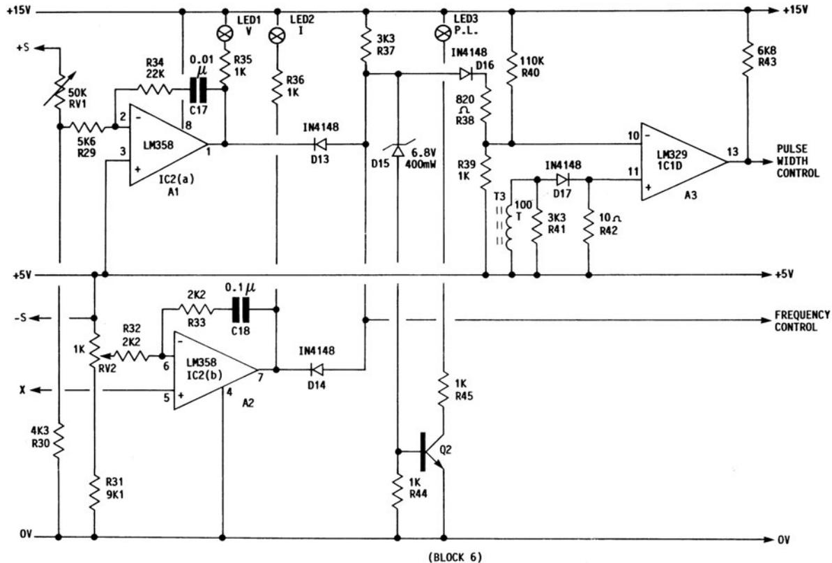
FIG. 2.24.6 Voltage and current control amplifiers for VSMPS.
