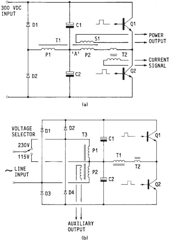
**FIG. 3.10.11** (a) A DC charge restoration circuit using an ancillary winding on the main switching transformer. DC restoration is required for current-mode-controlled half-bridge converters. (b) A DC charge restoration circuit using a center-tapped winding on the 60-Hz auxiliary transformer to restore the C1, C2 center point voltage.
