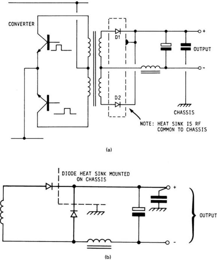
**FIG. 1.4.4** A method of reducing parasitic RFI currents in chassis-mounted output diode heat sinks by fitting the output choke in the common return line. (*a*) Push-pull applications; (*b*) single-ended outputs.
