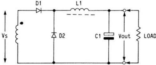
FIG. 2.9.3 Output filter of single-ended (buck-derived) forward converter.
