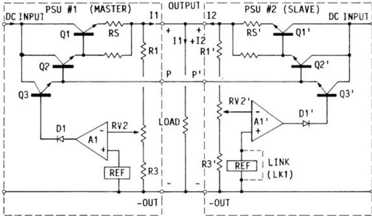
FIG. 1.24.1 Linear voltage-stabilized power supplies in master-slave connection.
