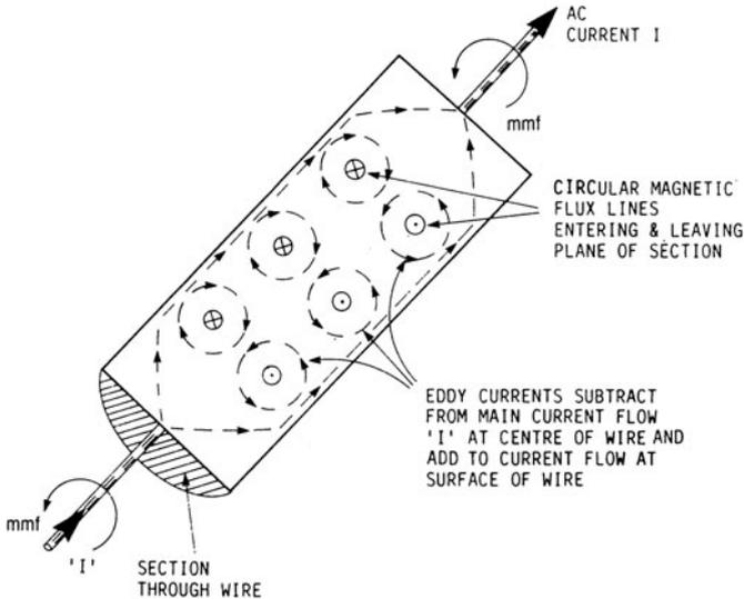
**FIG. 3.4B.2** Showing how "skin effect" is caused. Current is constrained to flow in the surface layer of the conductor as a result of concentric magnetic fields in the body of the conductor caused by the current flow.
