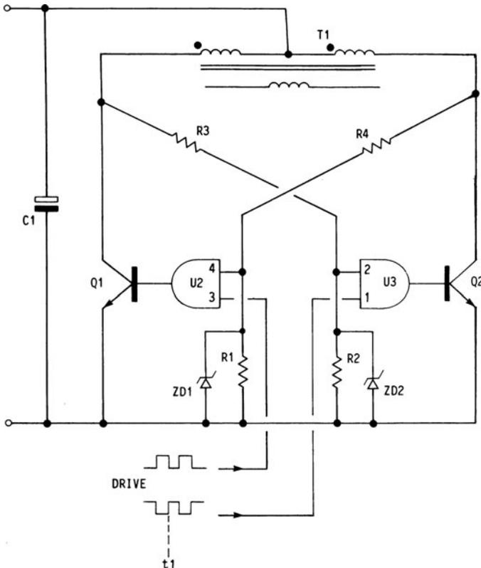
FIG. 1.19.3 Example of a cross-coupled cross-conduction inhibit circuit.
