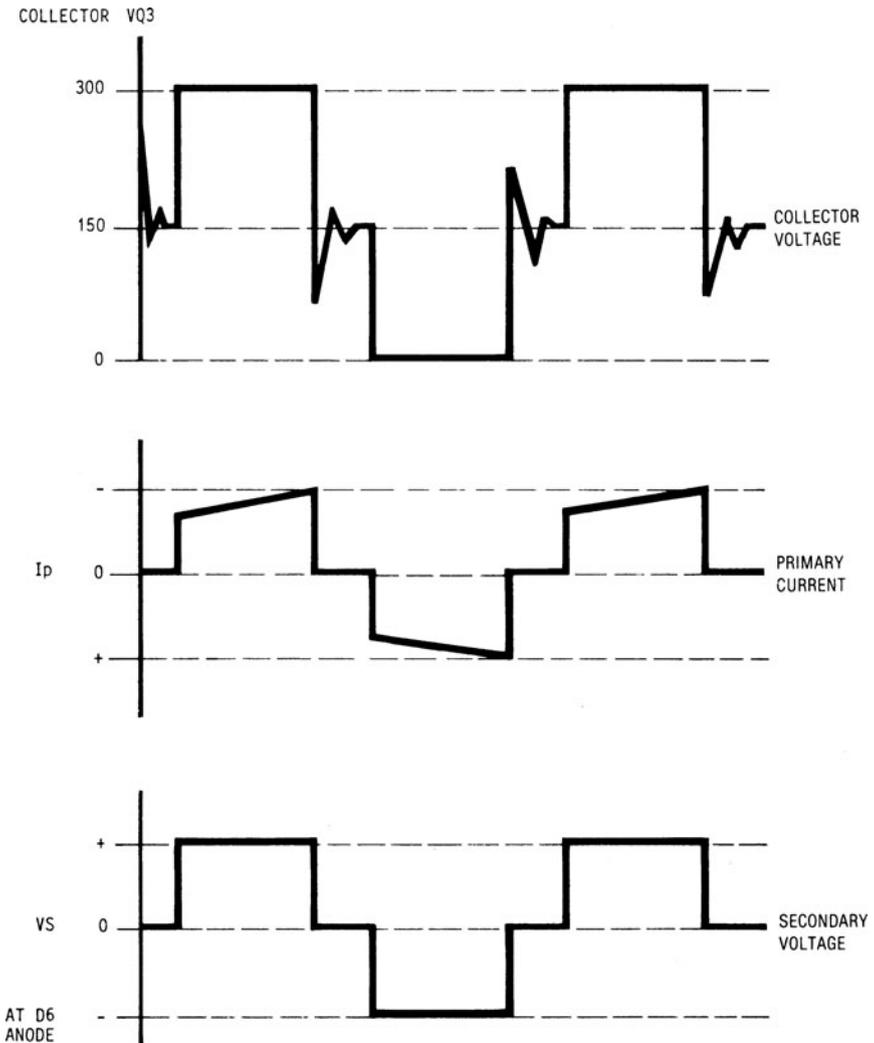
FIG. 2.13.2 Voltage and current waveforms for full-bridge converter.
