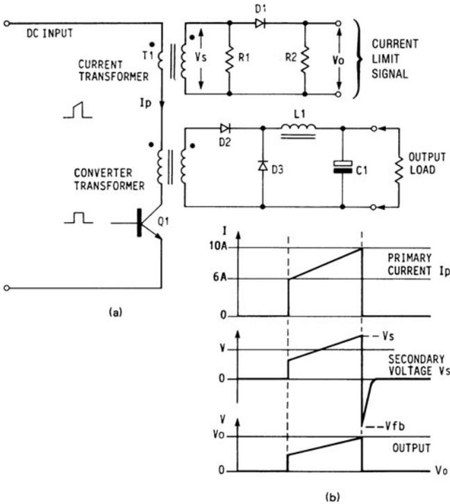
**FIG. 3.14.2** (a) Basic circuit of a single-ended forward converter, showing a unidirectional current transformer in the primary of the main power transformer. (b) Primary current and secondary voltage waveforms of current transformer, together with the current analogue signal voltage developed across R2. This may be used for current-mode control and current limiting.
