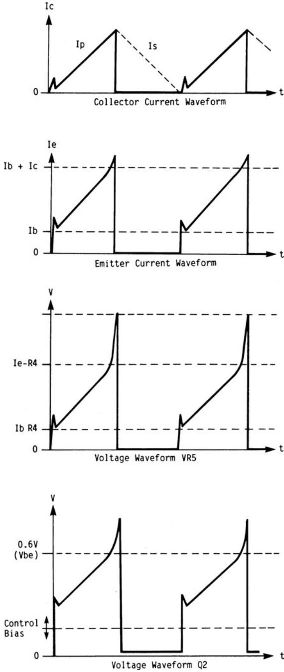
FIG. 2.7.1 Current and voltage waveforms of self-oscillating converter.
