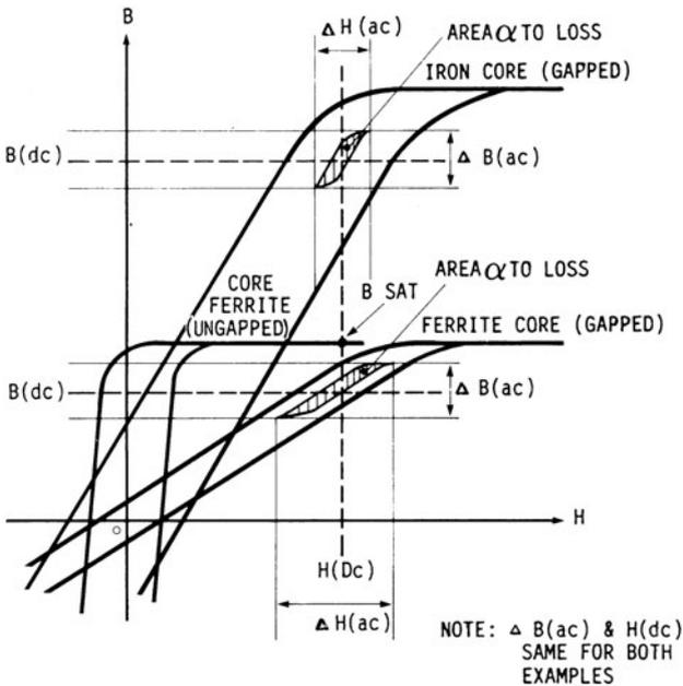
**FIG. 3.1.5** Comparison of the  $B/H$  characteristics of ferrite and iron cored chokes, with and without air gaps, showing the change in magnetizing current swing (ripple current) as a function of a fixed flux density swing (ripple voltage) for the two materials.
