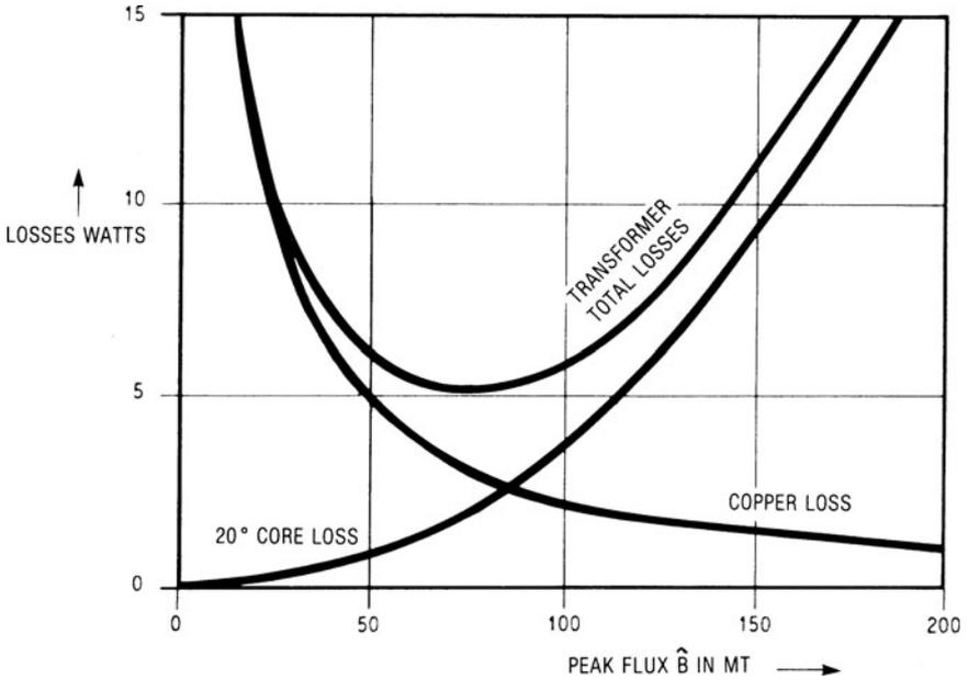
**FIG. 2.13.5** A16 ferrite core loss, copper loss, and total loss for a pair of EE55/55/21 cores, when wound for optimum performance in a typical switchmode transformer. Loss is shown as a function of the peak flux density. Note that in this example the minimum total loss occurs when the transformer induction (turns) is optimized so that the core loss is 44% of the total loss; however, at 50% the total loss is nearly the same.
