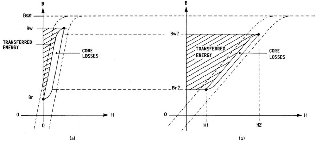
**FIG. 2.1.6** (a) Magnetization loop and energy transferred in a flyback converter transformer when the core air gap is small (high-permeability magnetic path). (b) Magnetization loop and energy transferred in a flyback converter transformer when a large air gap is used in the core.
