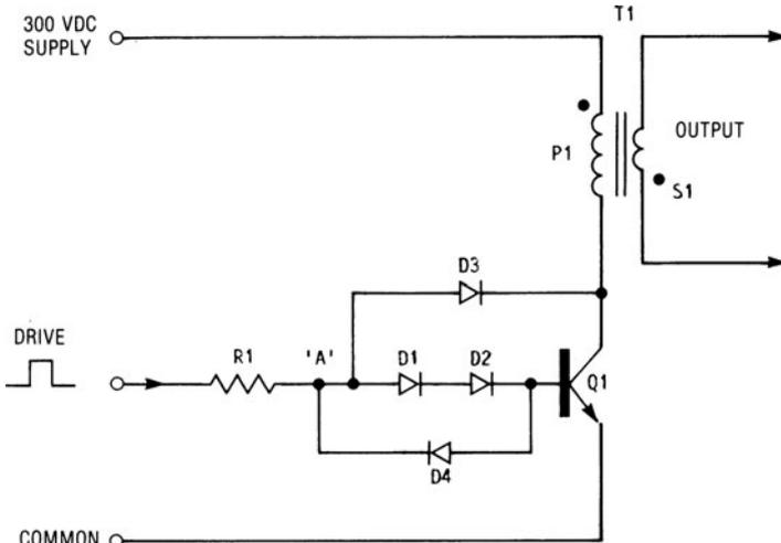
FIG. 1.17.1 "Baker clamp" antisaturation drive clamp circuit.
