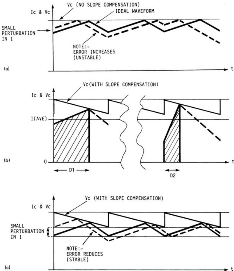
**FIG. 3.10.7** Current waveforms for continuous-inductor-current buck-derived converters, showing (a) subharmonic instability at duty ratios exceeding 50%. (b), (c) Also shown is the corrective effect of slope compensation in current-mode control.
