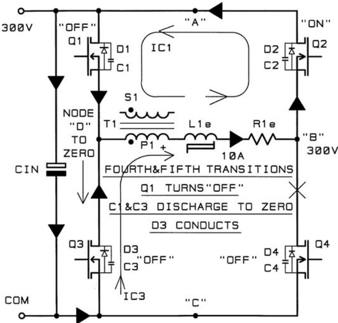
**FIG. 4.3.9** Shows the fourth transition, where Q1 turns "off" under ZVS conditions because the voltage at node "D" is 300 volts. Current continues to flow left to right via P1,  $L_{1e}$ , and  $R_{1e}$  as shown, discharging C1 and C3, and taking node "D" towards zero volts.
