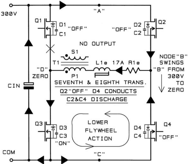
**FIG. 4.3.11** Shows the seventh and eighth transitions. In the seventh transition Q2 turns "off" under ZVS, because node "B" is at 300 volts. Current continues in  $L_{1e}$  from right to left as shown, and capacitors C2 and C4 discharge, taking node "B" towards zero.
