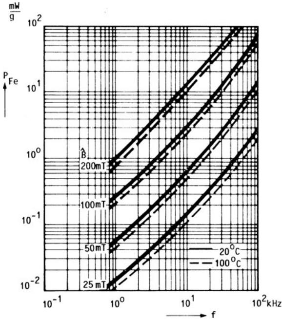
FIG. 2.13.4 Core loss per gram of A16 ferrite as a function of frequency, with peak flux density as a parameter. (Note: Graph is plotted for peak flux density  $\hat{B}$ ; flux density sweep  $IB$  is  $2 \times \hat{B}$ .) (Courtesy of Mullard Ltd.)
