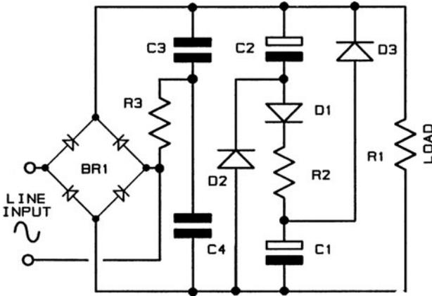
FIG. 4.1.9 An improved “valley-fill” circuit. (Spangler and Kit Sum.<sup>20, 85</sup>)
