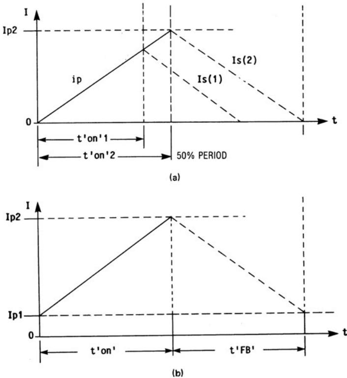
FIG. 2.1.5 (a) Primary current waveform  $I_p$  and secondary current waveforms  $I_s$  (discontinuous-mode operation). (b) Primary and secondary waveforms at the transition from the discontinuous mode to the continuous or incomplete energy transfer mode.
