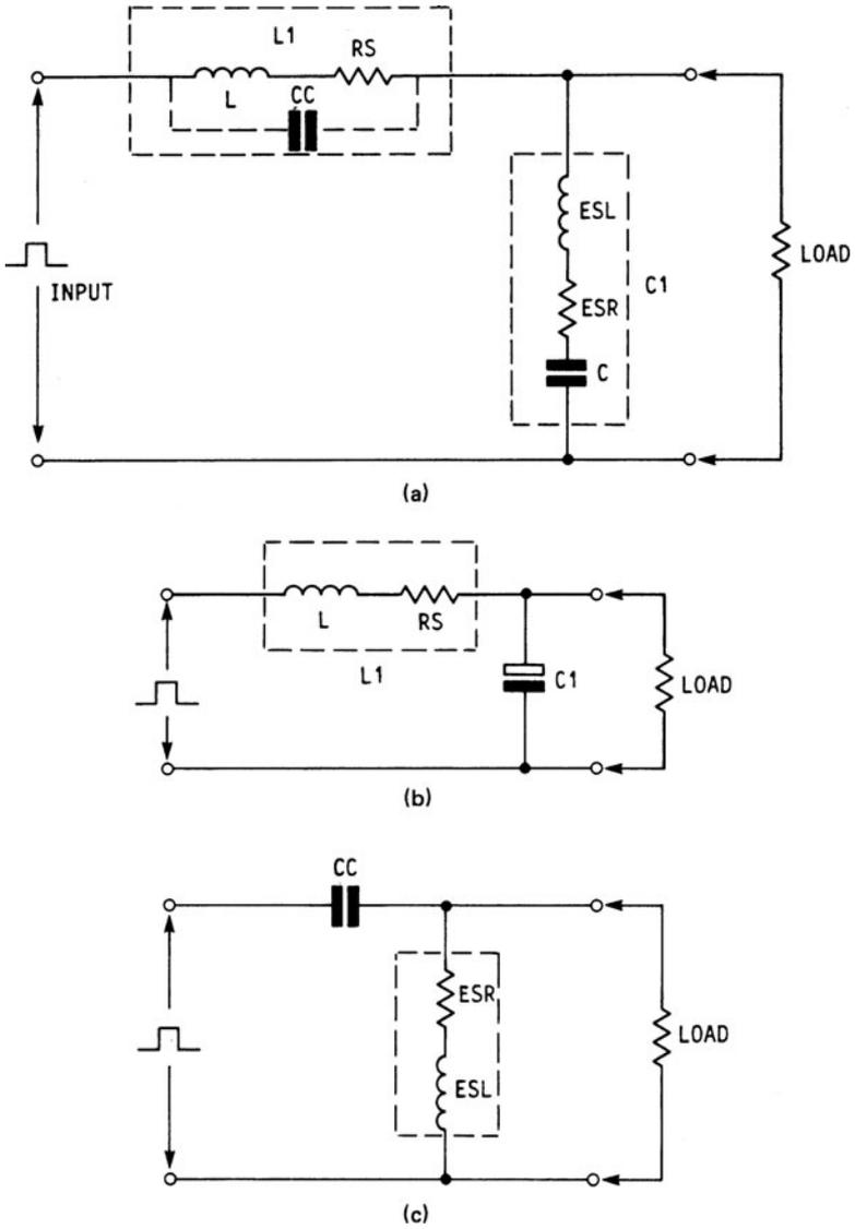
FIG. 1.20.1 (a) Power output filter, showing parasitic interwinding capacitance  $C_C$  and series resistance  $R_s$  for  $L1$ , and series inductance  $ESL$  and resistance  $ESR$  for  $C1$ . (b), (c) Output filter equivalent circuits at low frequency (b) and high frequency (c).
