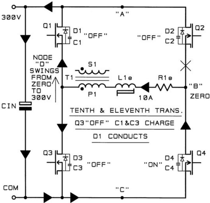
**FIG. 4.3.13** Shows the tenth and eleventh transitions. At the tenth transition, Q3 turns “off” under ZVS conditions because node “D” is at zero volts. C3 and C1 now charge up, taking node “D” to 300 volts. At the eleventh transition, D1 conducts and clamps node “D” at 300 volts, and Q1 is ready to be turned “on” under ZVS conditions.
