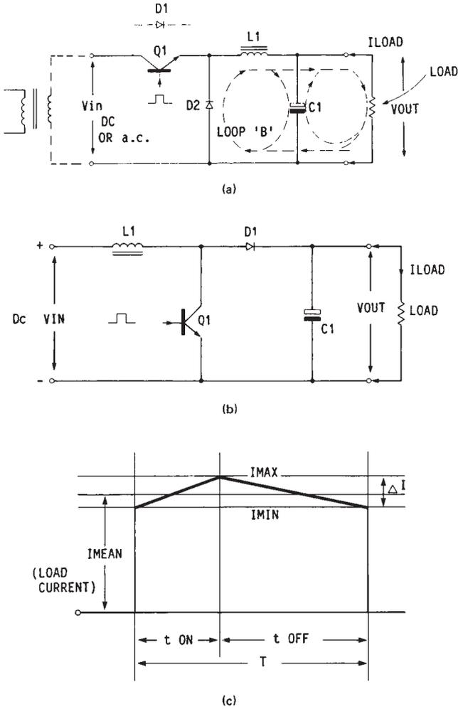
**FIG. 3.1.6** (a) Basic buck regulator circuit. (b) Basic boost regulator circuit. (c) Output current waveform for buck regulator and input current waveform for boost regulator, with  $L1$  in continuous-mode conduction.
