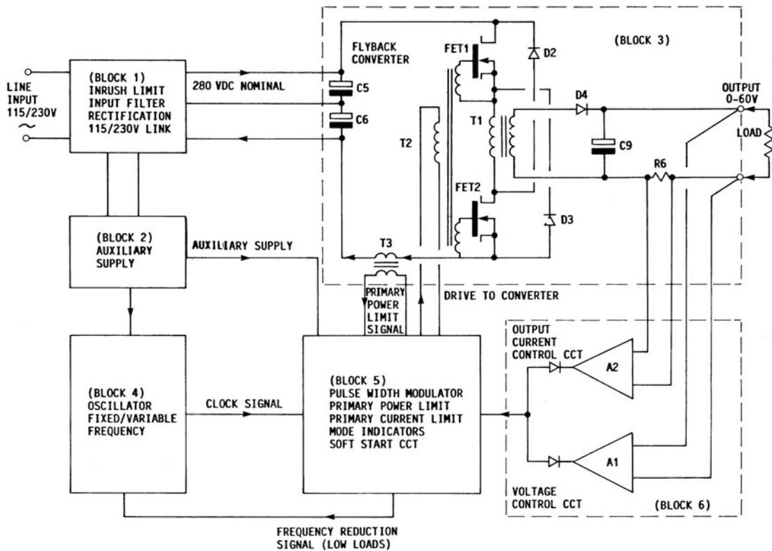
FIG. 2.24.3 Block diagram of variable switchmode power supply.
