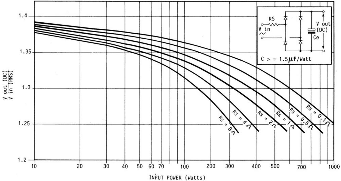
FIG. 1.6.7 Mean DC output voltage of a full-wave bridge-rectified capacitor input filter as a function of load power, with effective source resistance as a parameter. (Valid for capacitor values of  $1.5 \mu F/W$  or greater.)
