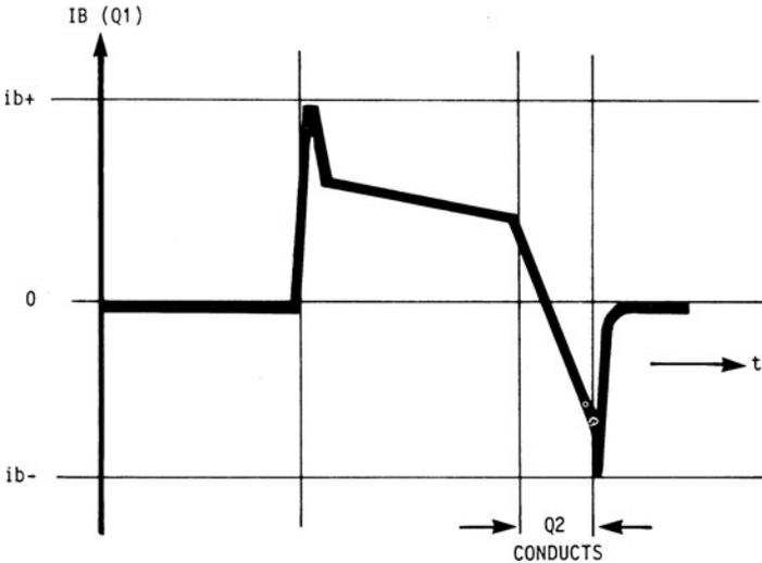
FIG. 2.6.3 Base drive current waveform of self-oscillating converter.
