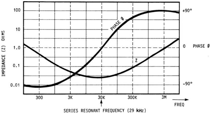
**FIG. 1.20.4** Impedance and phase shift of a typical commercial-grade 470- $\mu\text{F}$  electrolytic capacitor as a function of frequency. Note self-resonant frequency and minimum impedance at 29 kHz.
