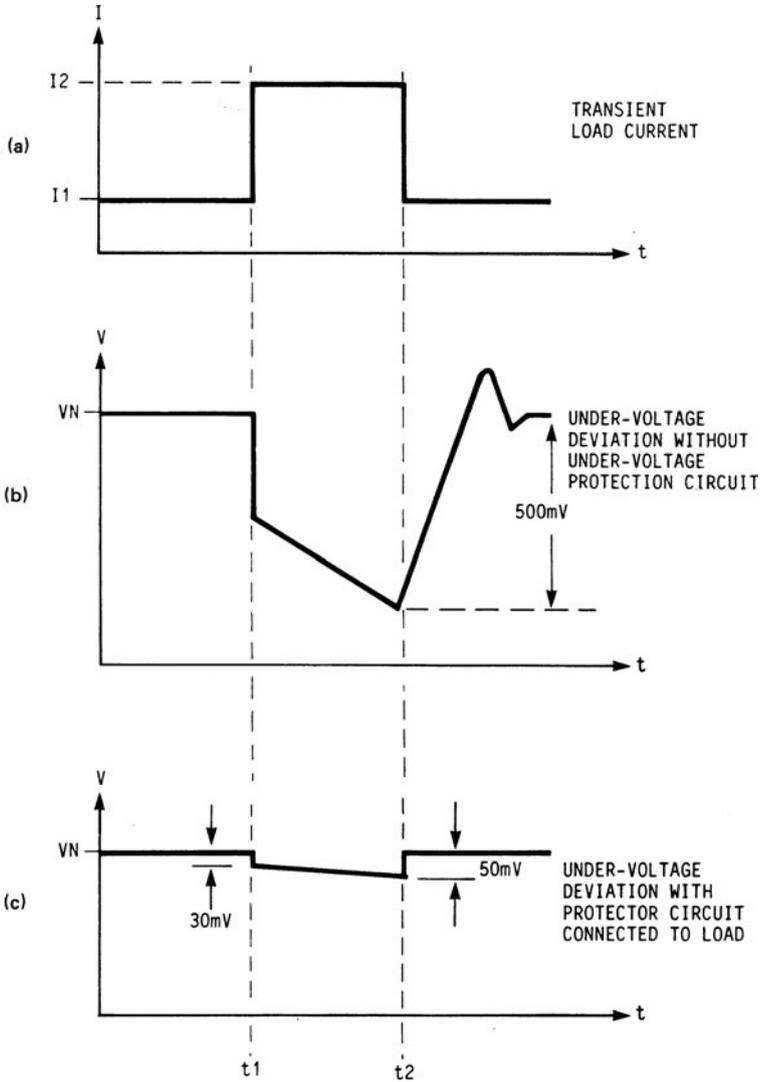
**FIG. 1.12.1** Characteristics of atypical "undervoltage transient protection" circuit. (a) Load current transient. (b) Typical undervoltage transient excursion without protection circuit fitted. (c) Undervoltage transient excursion with protection circuit fitted.
