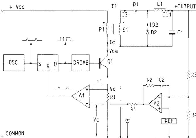
FIG. 3.10.5 Forward converter (buck-derived), with closed-voltage-loop current-mode control.
