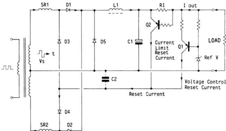
FIG. 2.21.9 Push-pull saturable reactor secondary regulator circuit.
