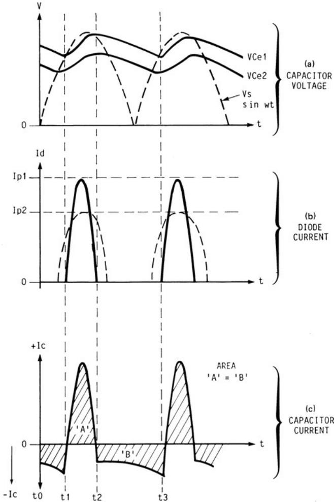
**FIG. 1.6.3** Rectifier and capacitor voltage and current waveforms in a full-wave capacitor input filter. (a) Capacitor voltage waveform; (b) rectifier diode current waveform; (c) capacitor current waveform.
