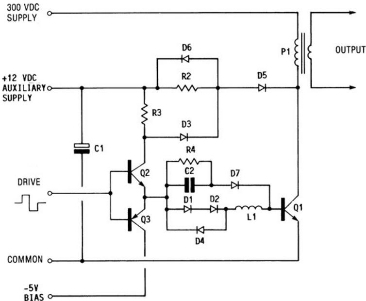
FIG. 1.18.4 Snubber diode and Baker antisaturation clamp combination.
