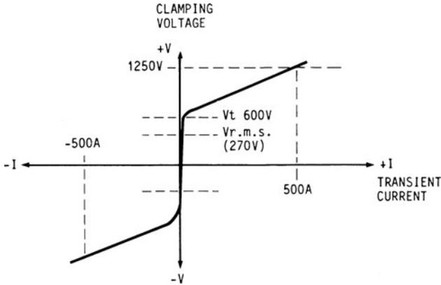
FIG. 1.2.5 Metal oxide varistor (MOV) performance characteristics.
