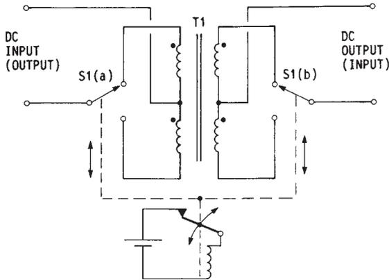
**FIG. 2.17.1** DC-to-DC transformer (mechanical synchronous vibrator type).
