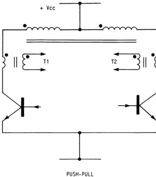
**FIG. 3.6.1** Basic push-pull power circuit, showing current transformer locations (T1 and T2) for forced flux density balancing in push-pull topologies.
