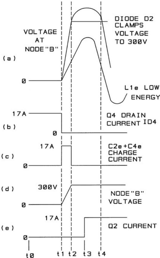
**FIG. 4.3.7** Shows the voltage and current waveforms during the first two transitions.
