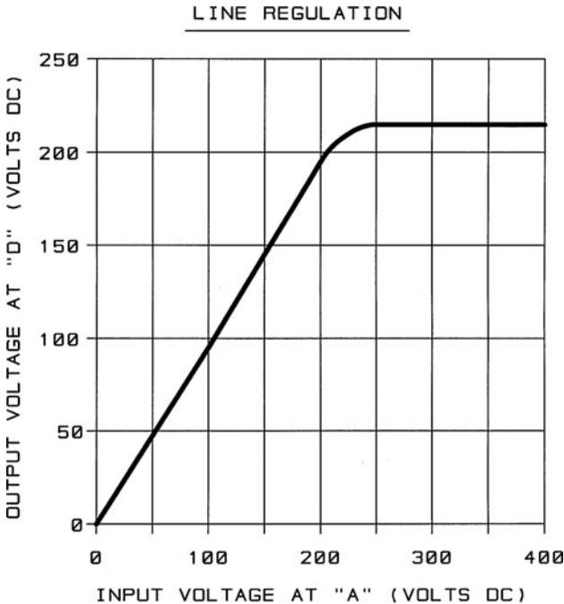
**FIG. 1.23.6** shows the DC voltage regulation at the output of the linear regulator at node "D," for input voltages measured at node "A" in the range zero to 400 volts. Notice the linear transfer ratio from zero to 250 volts, followed by good output regulation at 215 volts for inputs from 250 to 400 volts DC. The characteristic provides a good low-voltage start up action for the 50 kHz sine wave inverter section shown in Fig. 1.23.8, and good voltage regulation over the working range.
