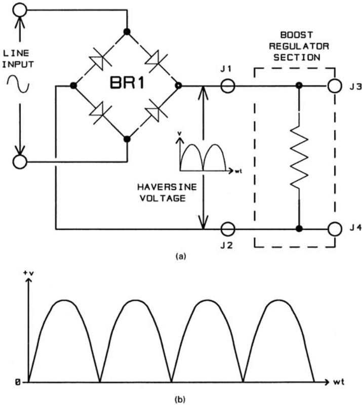
**FIG. 4.1.11** (a) Bridge rectifier (without capacitor) used at the line input to produce a haversine voltage waveform at the input to an active power factor correction system. (b) A typical haversine voltage waveform.
