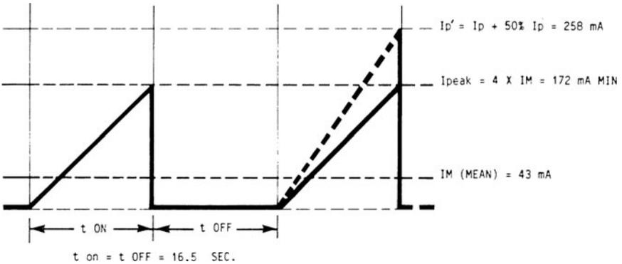
FIG. 2.14.2 Primary current waveform for self-oscillating auxiliary converter.
