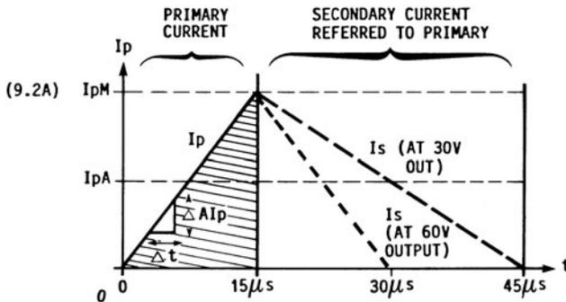
FIG. 2.25.1 Current waveform in discontinuous mode.
