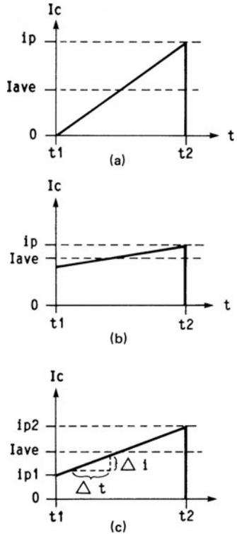
**FIG. 2.2.4** Primary current waveforms in flyback converters. (a) Complete energy transfer mode; (b) incomplete energy transfer mode (maximum primary inductance); (c) incomplete energy transfer mode (optimum primary inductance).
