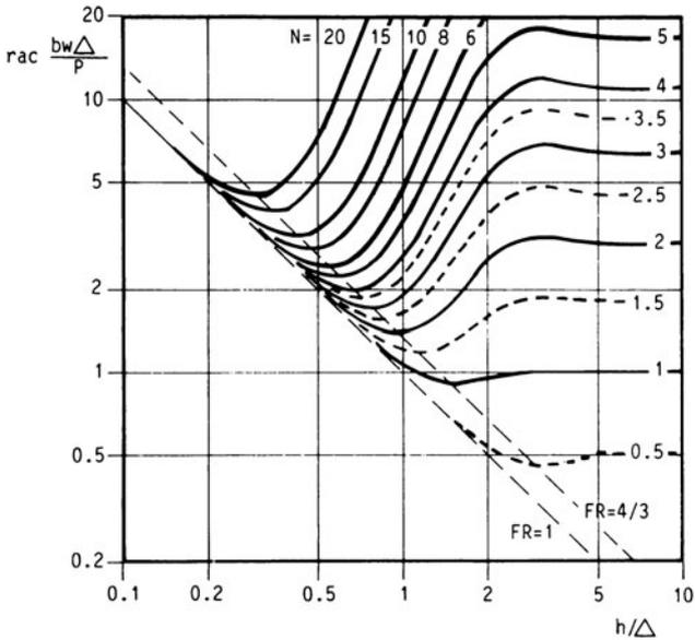
**FIG. 3.4B.5** Plot of  $R_{ac} b_w \Delta / \rho$  with number of layers as a parameter, showing the development of the conditions for optimum  $F_r$  ratio and optimum conductor thickness. (*J. Jongsma 1882 Mullard Ltd. Ref. 58.*)
