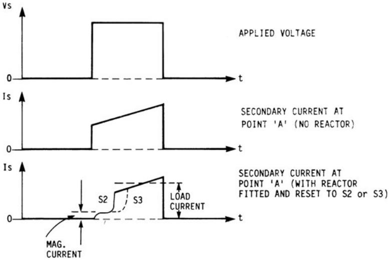
FIG. 2.21.6 Secondary current waveforms with saturable reactor fitted.
