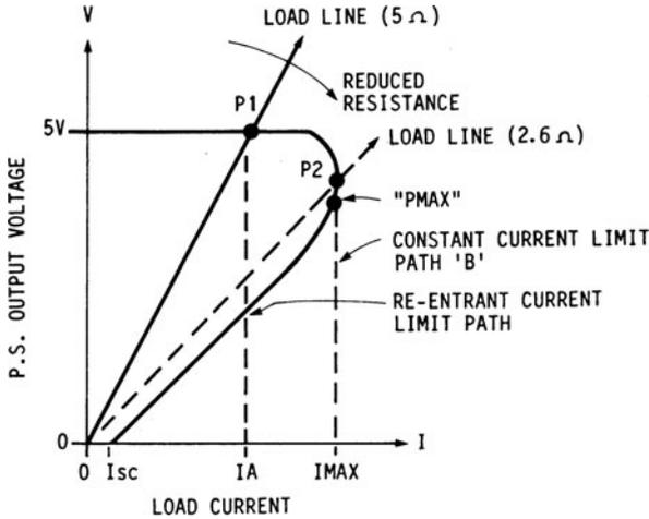
FIG. 1.14.1 Current overload reentrant shutdown characteristic of fold-back current-limited supply.
