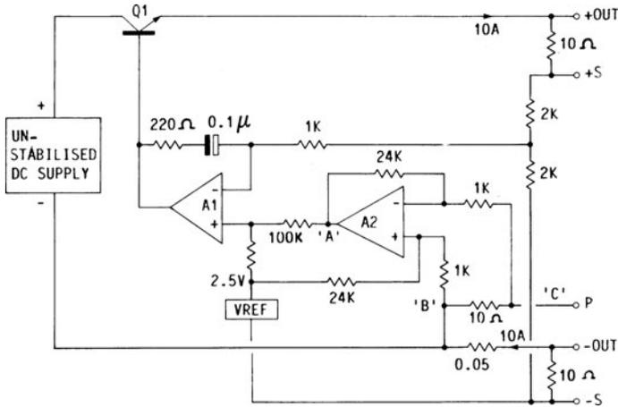
FIG. 1.24.4 Example of a forced current-sharing circuit.
