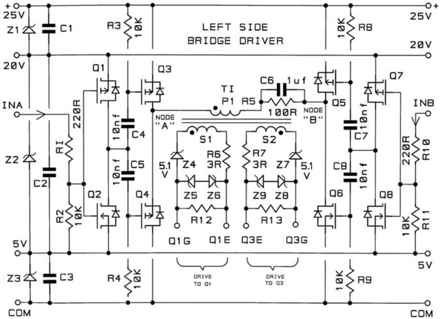
**FIG. 4.3.22** Shows a more powerful drive interface, suitable for high power applications. The FETs used in the 5-kW application have gate input capacitance  $C_{iss}$  of 20 nF, and a low resistance gate drive is required for fast switching.
