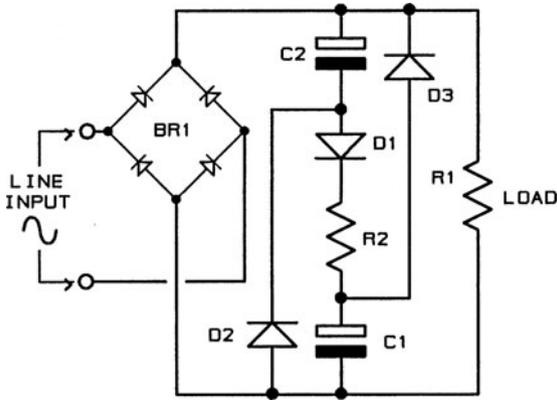
FIG. 4.1.7 "Valley-fill" power factor correction circuit used in low-power applications. (Spangler.<sup>86</sup>)
