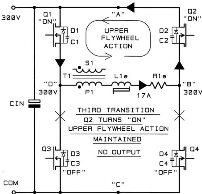
**FIG. 4.3.8** Shows the third transition where Q2 turns "on" at  $t_3$  under zero voltage conditions. The upper loop flywheel current transfers from D2 to the drain-source of the FET Q2. The voltage across main transformer T1, primary P1, is near zero and energy is not being transferred to the output. The upper flywheel current loop continues with little loss as the loop resistance is quite small. This is the first "off" state of the bridge, and will continue for the "off" period.
