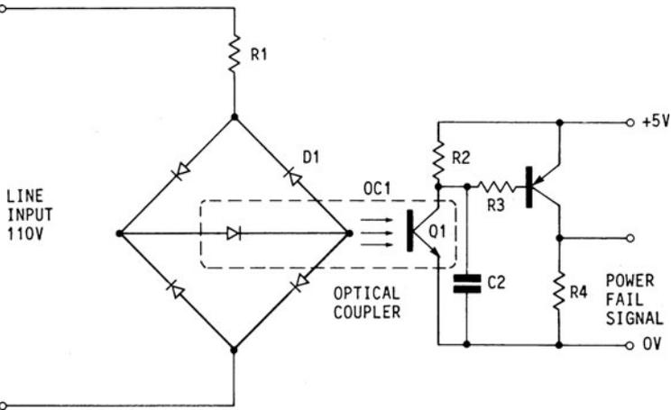
FIG 1.21.1 Simple optocoupled power failure warning circuit.
