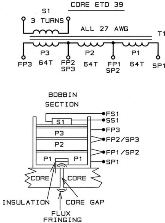
**FIG. 4.2.5** Shows how the transformer T1 should be made up. Notice in particular that the core is “butt-gapped;” that is, the gap spans all three legs. This is preferred to reduce the fringing that occurs when a larger gap appears in the center pole only. Flux fringing causes excessive local heating in the magnet wire near the gap. Also notice the build up of insulation in the area of the gap, done to prevent magnet wire being wound in close proximity to the core gap, for the same reason.
