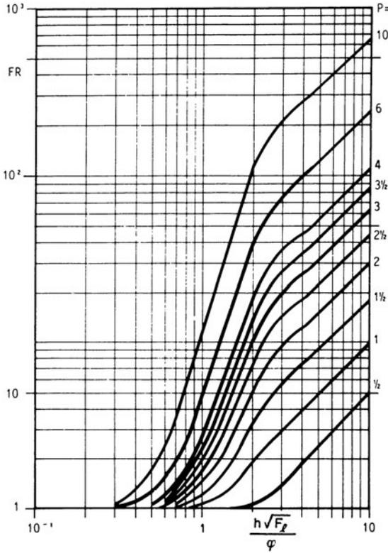
FIG. 3.4B.1  $F_r$  ratio (ratio of ac/DC resistance as a result of skin effect) as a function of the effective conductor thickness, with number of layers  $P$  as a parameter (After Dowell<sup>31</sup>.)
