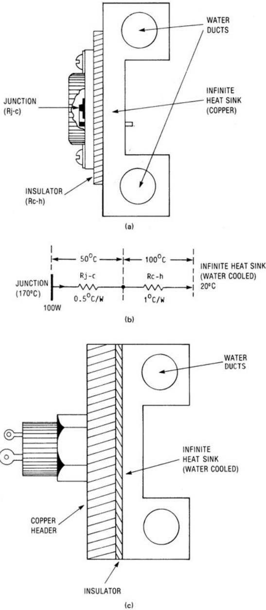
**FIG. 3.16.4** (a) Thermal resistance example, showing a T0-3 transistor mounted on a water-cooled (near-infinite) heat sink. (b) Equivalent thermal resistance circuit model for T0-3 transistor on "near infinite" heat sink. (c) T0-111 stud transistor on "near infinite" heat sink, with a copper header.
