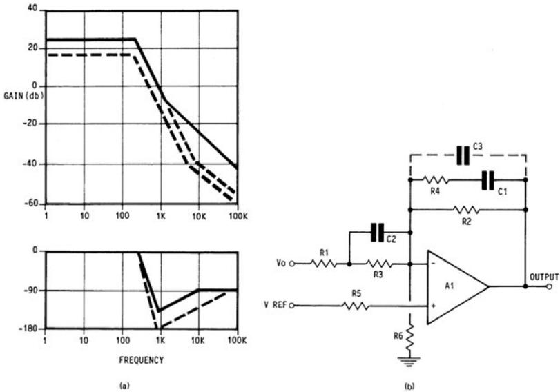
**FIG. 3.10.9** (a) Transfer function of the same converter using duty ratio control, showing the more complex two-pole response. (b) The compensation network required for the two-pole duty-ratio-controlled circuit.
