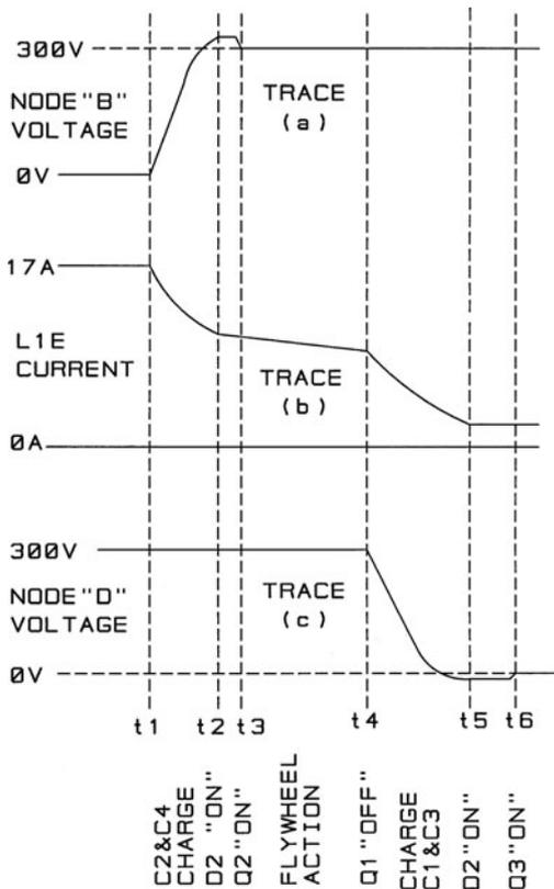
**FIG. 4.3.16** Shows the waveforms during the right side transition. Trace (a)  $t_1$  to  $t_2$  shows the node "B" ringing up to the voltage where D2 conducts. At  $t_3$ , Q1 turns "on" and the voltage at node "B" clamps to 300 volts.
