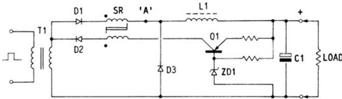
**FIG. 2.21.7** Two-winding saturable reactor regulator (transductor type) applied to buck regulator output circuit.
