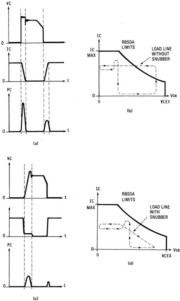
**FIG. 1.18.2** “Safe operating area” characteristics, with and without snubber circuits. (a) Turn-on and turn-off voltage, current, and dissipation stress without load line shaping. (b) Active load line imposed on “reverse base safe operating area” (RBSOA) limits without load line shaping. (Note secondary breakdown stress.) (c) Turn-on and turn-off voltage, current, and dissipation stress with load line shaping. (d) Load line and (RBSOA) limits with load line shaping.
