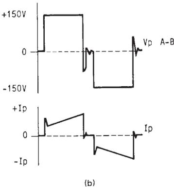
**FIG. 2.12.1** (a) Power section of half-bridge push-pull forward converter. (b) Collector voltage and current waveforms for half-bridge forward converter.
