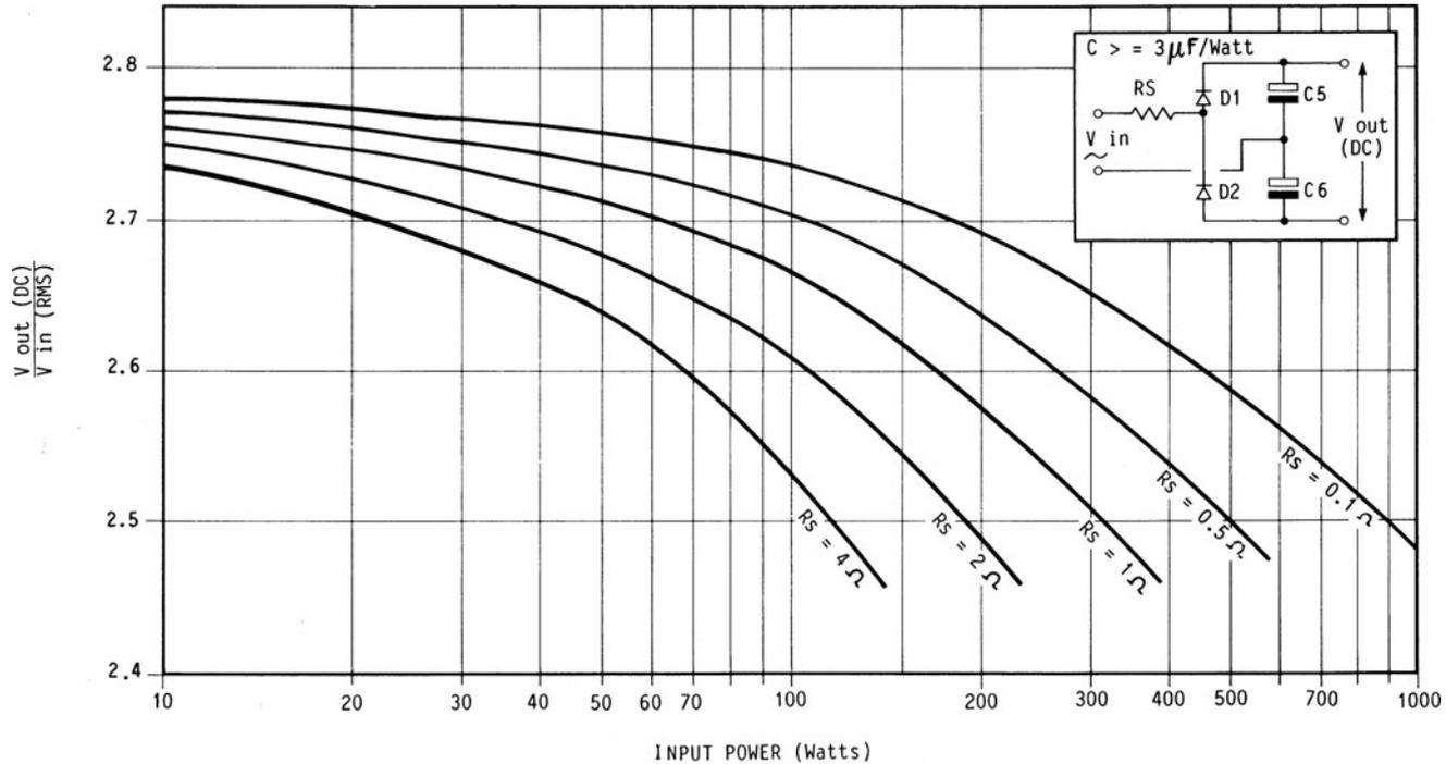
**FIG. 1.6.8** Mean DC output voltage of a voltage doubler capacitor input filter as a function of load power, with effective source resistance as a parameter. (Valid for capacitor values of  $3 \mu F/W$  or greater.)
