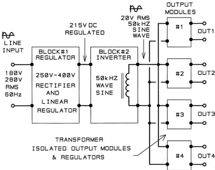
**FIG. 1.23.4** shows the block diagram of a regulated distributed ancillary power system intended to provide multiple, distributed and isolated auxiliary supplies to multiple control PCBs in a large power system. Sine wave power is distributed via two pin connectors and twisted pairs at 50 kHz, 20 volts. This provides for low-noise, semi-regulated local supplies on each PCB, using local, small, high-frequency transformers and secondary rectifiers.
