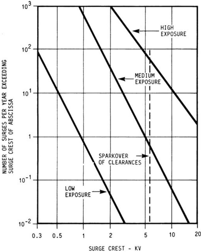
FIG. 1.2.2 Rate of surge occurrences versus voltage level at unprotected locations.
