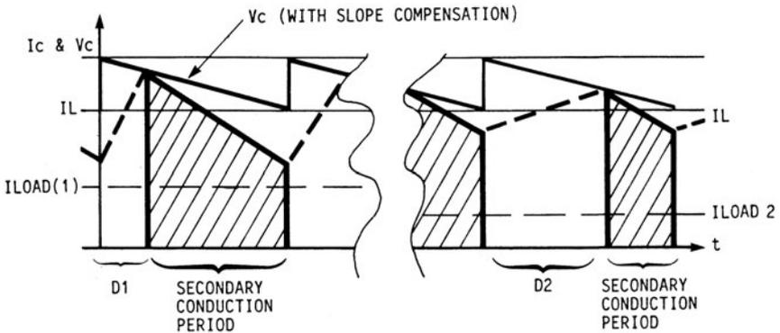
FIG. 3.10.10 Primary and secondary current waveforms of a boost converter, showing that the immediate effect of increasing the “on” pulse width from  $D1$  to  $D2$  is a reduction in the secondary conduction period, and hence the transferred energy (the cause of the right-half-plane zero).
