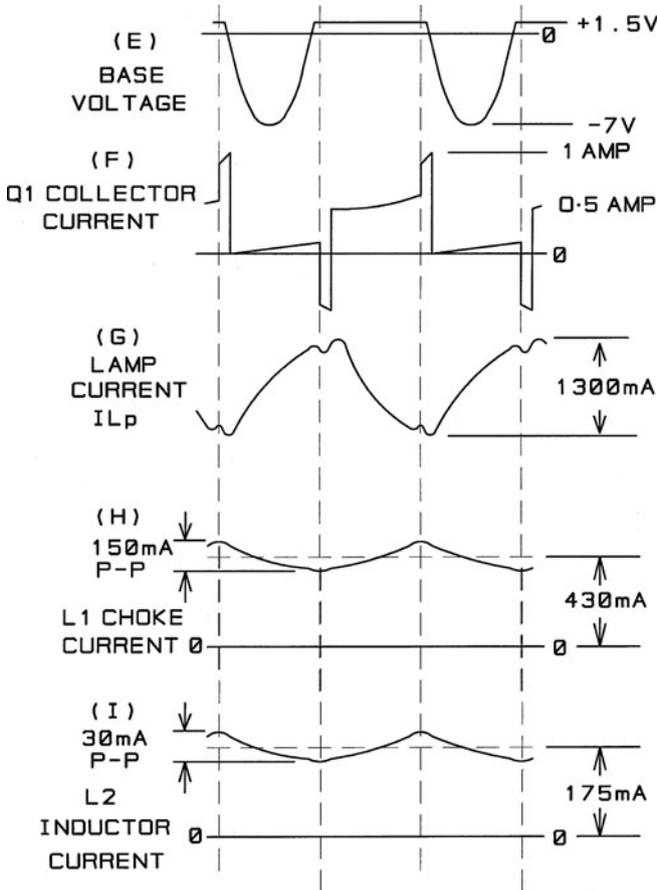
**FIG. 4.2.4** (E-I) shows the drive waveforms on the base of Q1 and Q2. Notice the large negative voltage swing used to establish the drive current in L2. Trace (F) shows Q1 and Q2 collector currents at full load. Trace (G) shows the lamp current, trace (H) the current in L1, and trace (I) the current in L2.
