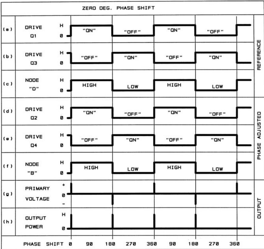
**FIG. 4.3.23** Shows the timing for the four power FET gate drive waveforms (without any allowance for switching delays). It also shows the node "B" and node "D" voltage waveforms for zero degrees phase shift.
