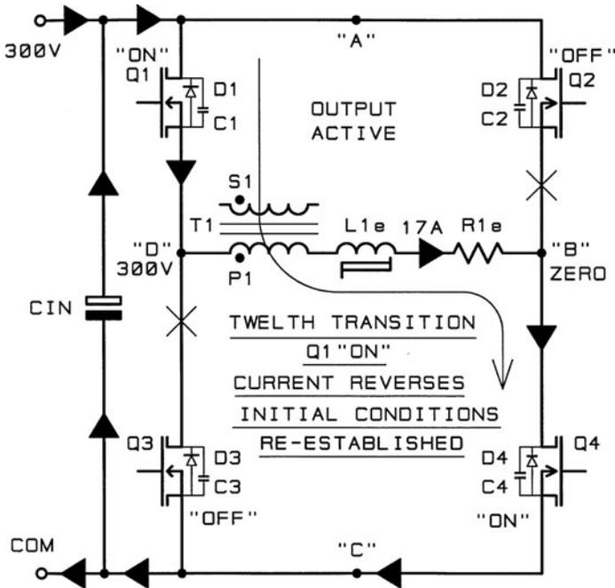
FIG. 4.3.14 Shows the twelfth transition where Q1 turns "on." The full supply voltage now appears across P1,  $L_{1e}$ , and  $R_{1e}$ , and the current quickly reverses again and flows as shown. This returns us to the starting condition, with power being transferred to the output as shown in Fig. 4.3.3.
