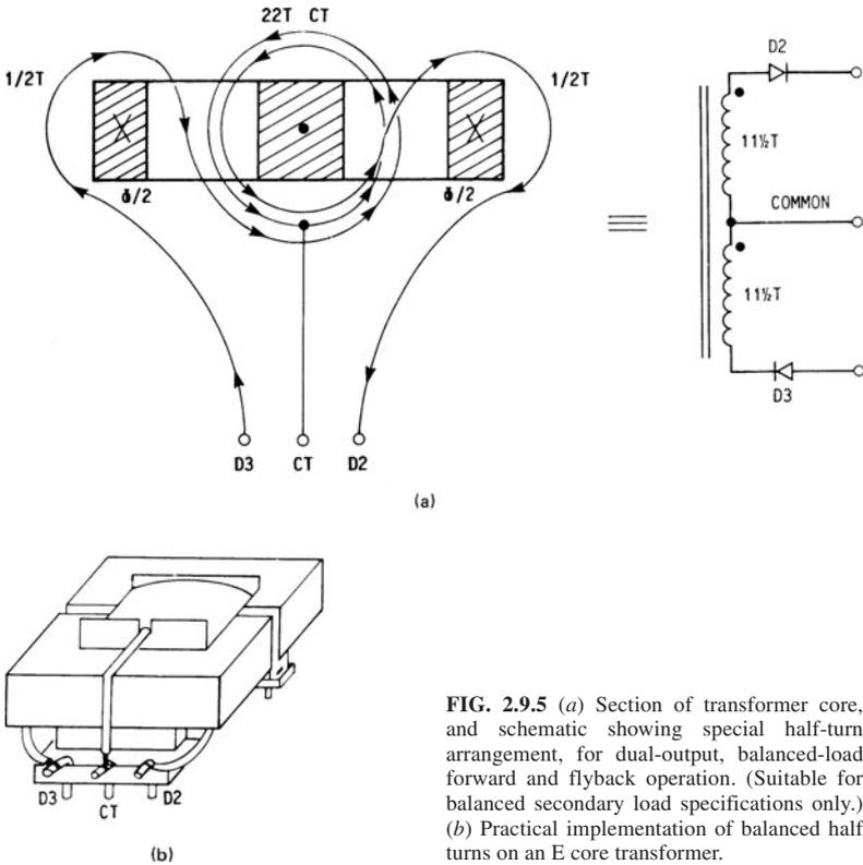
**FIG. 2.9.5** (a) Section of transformer core, and schematic showing special half-turn arrangement, for dual-output, balanced-load forward and flyback operation. (Suitable for balanced secondary load specifications only.) (b) Practical implementation of balanced half turns on an E core transformer.
