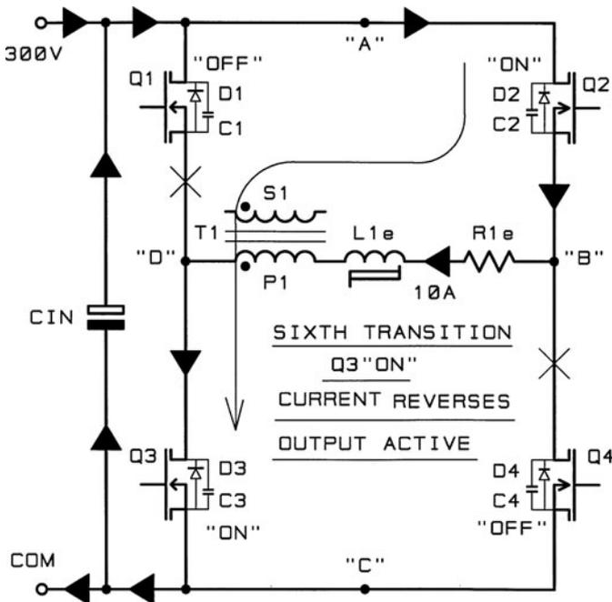
FIG. 4.3.10 Shows the sixth transition with Q3 turned "on." The current has reversed and flows right to left via Q2,  $R_{1e}$ ,  $L_{1e}$ , P1, and Q3 as shown. The voltage across P1 has reversed, and the full supply voltage is applied. Power is again being delivered to the output. This is the second "on" period and is maintained for the required "on" period.
