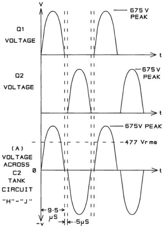
**FIG. 1.23.10** shows the waveforms expected across the tank circuit (the voltage across C2) node "H" to node "J." (A similar voltage will be found across the output winding S2, but the amplitude will be much smaller).
