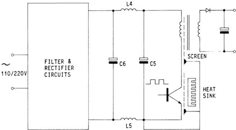
FIG. 1.3.5 Preferred positions for primary-to-ground-plane RFI screens.
