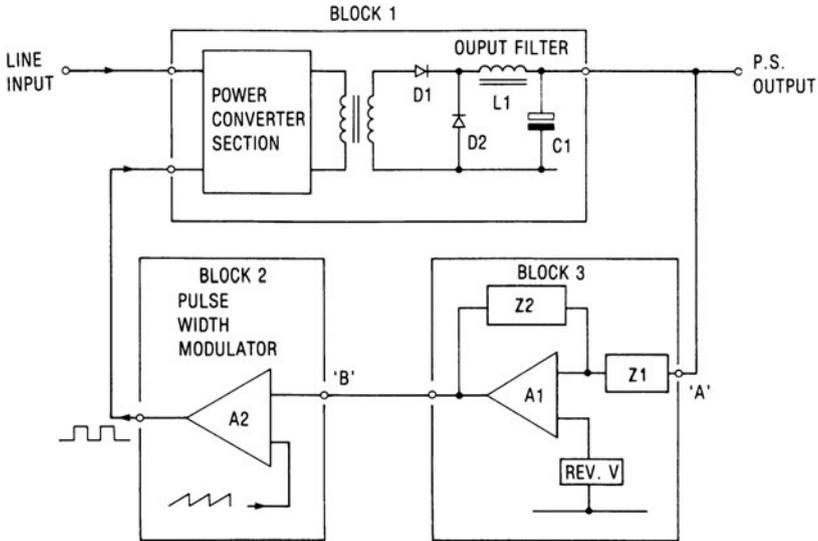
**FIG. 3.8.1** Block schematic diagram of the control loop, for a forward (buck-derived) switchmode power converter. Showing power section block 1, pulse-width modulator block 2, and control circuit block 3.
