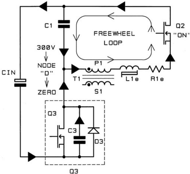
FIG. 4.3.17 Shows the active components during a left side transition. During the period when node "D" is dropping from 300 volts to zero, half the current now left in  $L_{1e}$  flows in C1 and the other half in C3.
