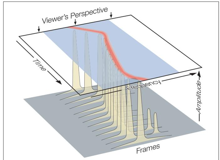
**Figure 3-2.** Spectrogram display.
