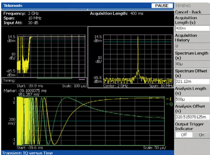
Figure 3-10. IQ vs. Time measurement of settling transient.
