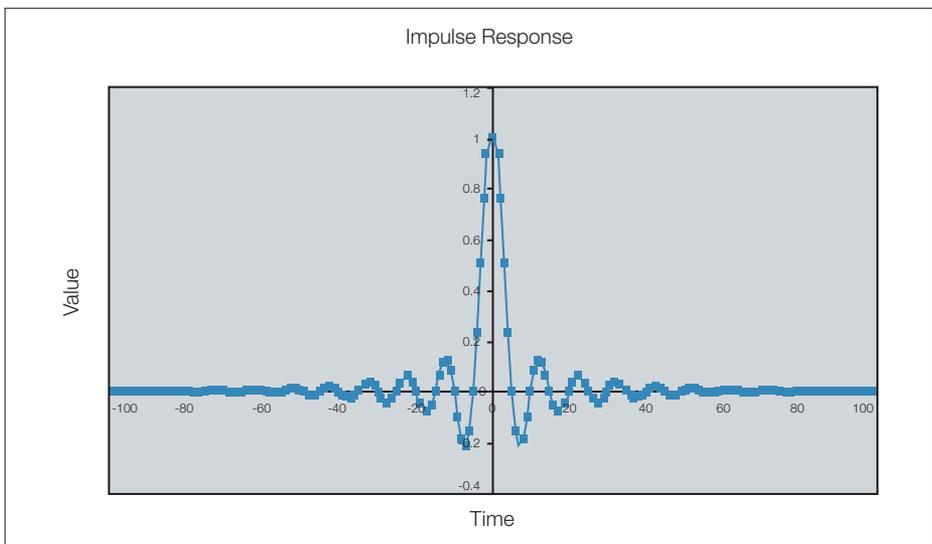
Figure 2-16. Impulse response for the lowpass filter in Figure 2-15.
