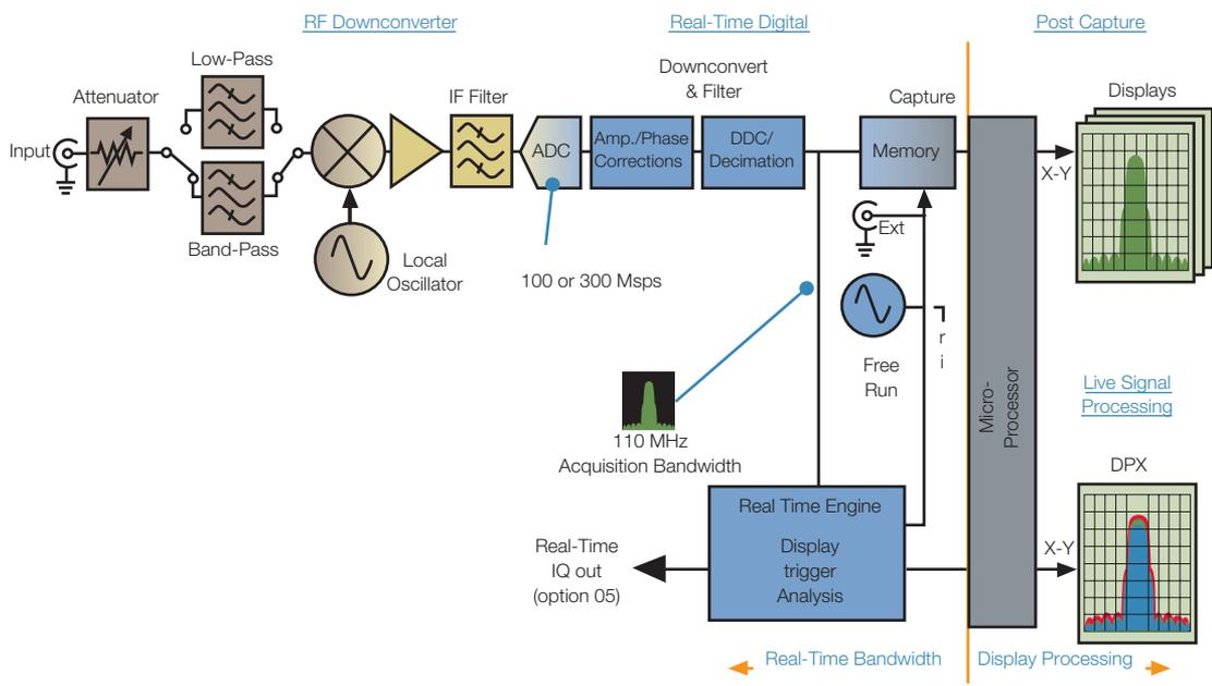
c) Real-Time Spectrum Analyzer (RSA6100 Series + Option 110)
