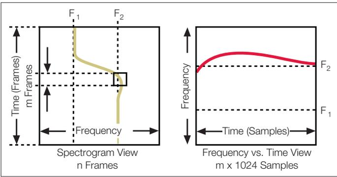
Figure 3-5. Comparison of spectrogram and Frequency vs. Time.
