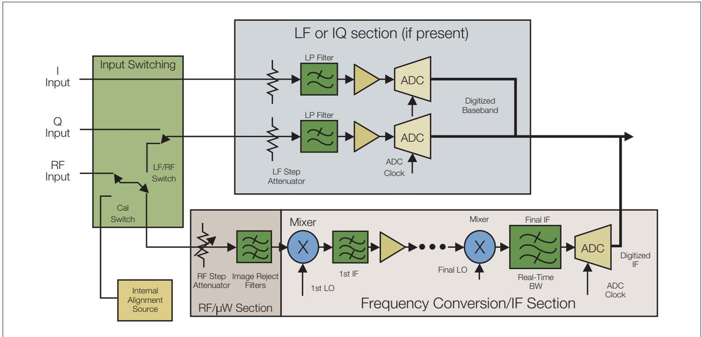
Figure 2-1. Real-Time Spectrum Analyzer RF/IF block diagram.
