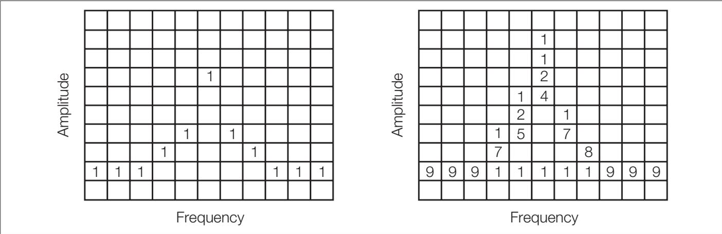
Figure 2-21. Example 3-D Bitmap Database after 1 (left) and 9 (right) updates. Note that each column contains the same total number of hits.
