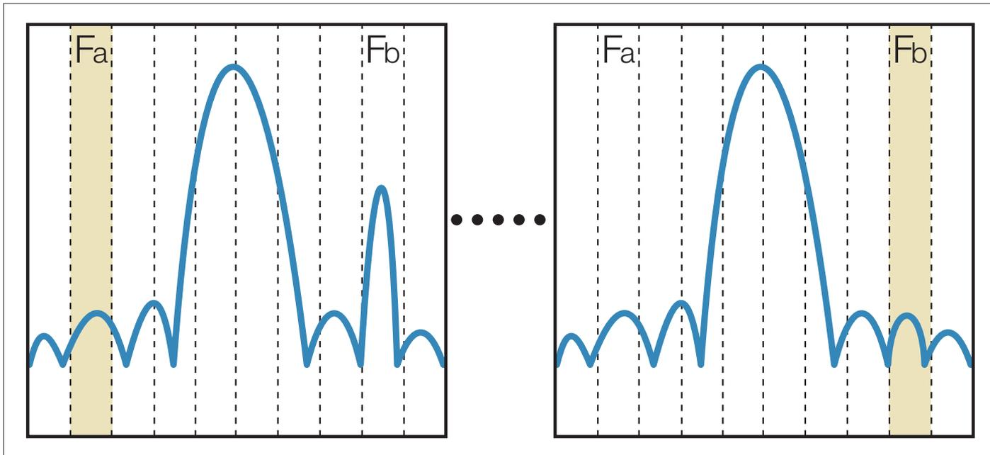
**Figure 1-1.** The Swept Spectrum Analyzer steps across a series of frequency segments, often missing important transient events that occur outside the current sweep band highlighted in tan segment Fb on the right.
