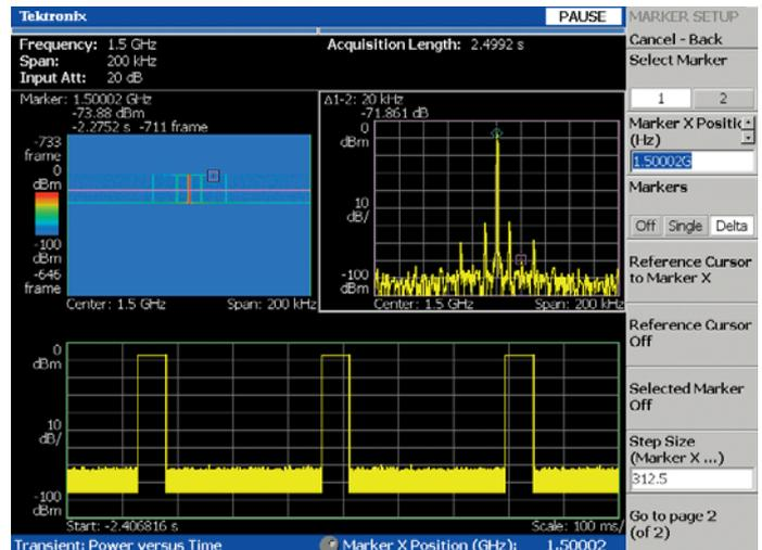
Figure 3-24. Multi-domain view showing Spectrogram, power vs. frequency, and power vs. time.
