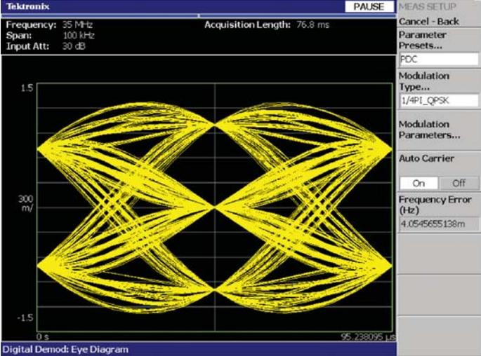
Figure 3-16. Eye diagram display showing a PDC signal.
