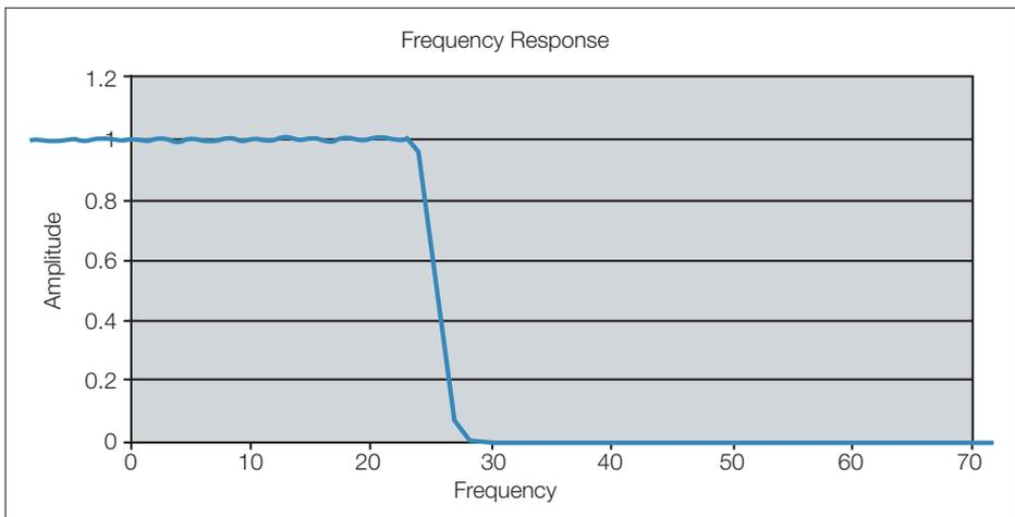
Figure 2-15. Frequency response of a lowpass filter.
