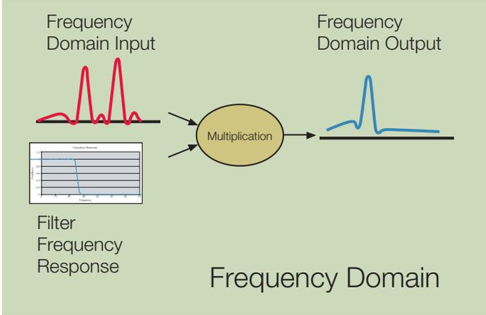
Figure 2-17. Multiplying a filter by its frequency response.
