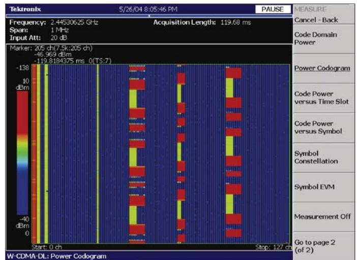
Figure 3-20. Codogram measurement of W-CDMA compressed mode.
