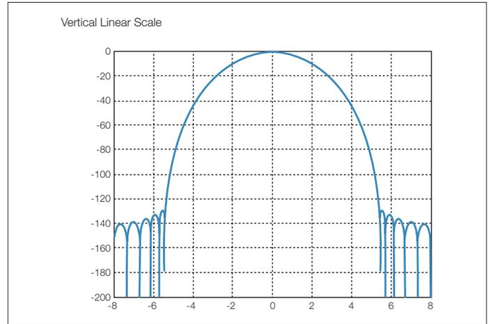
**Figure 2-10.** The spectrum of a Kaiser window (beta 16.7). The horizontal scale unit is the frequency bin ( $F_c/N$ ). The vertical scale is in dB.
