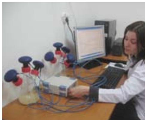
*Fermentation Process monitoring with CO<sub>2</sub>-Ethanol-O<sub>2</sub> sensors*
