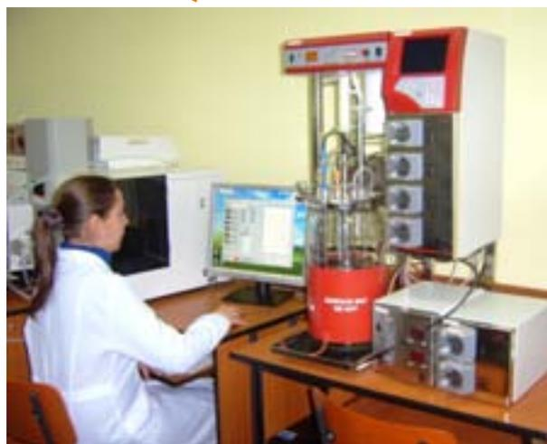
*Computer Controlled Bioreactor*
