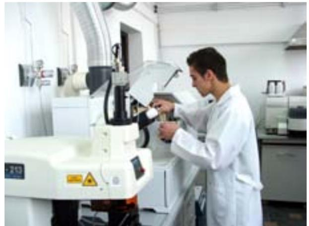
*Atomic Emission Spectrometer with Mass Spectrometer and Laser Ablation*
