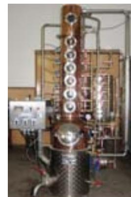
*Computer Controlled Distilling column*
