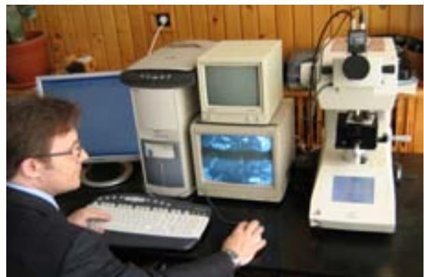
*Vickers Microdurimeter controlled by computer*
