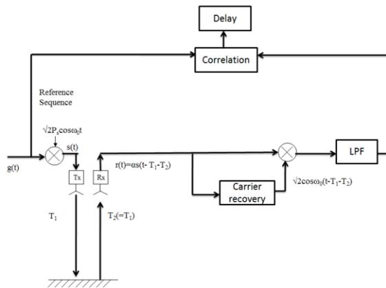
Fig.1. Ranging Using DS Spread Spectrum
