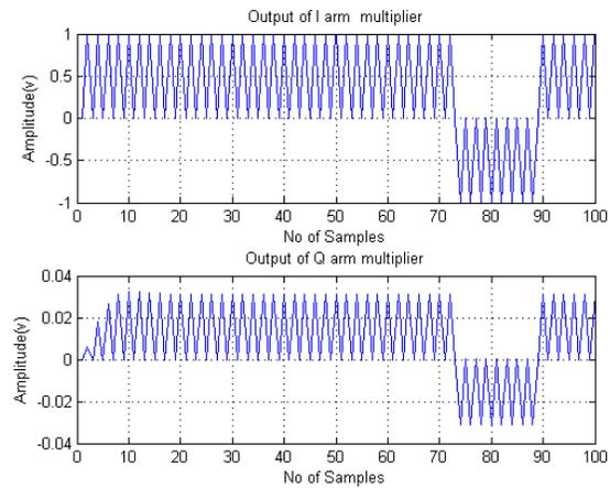
Fig.6. Outputs of I-arm and Q-arm multiplier
