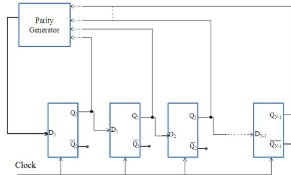
Fig.1. Maximum Length PN Sequence Generator
