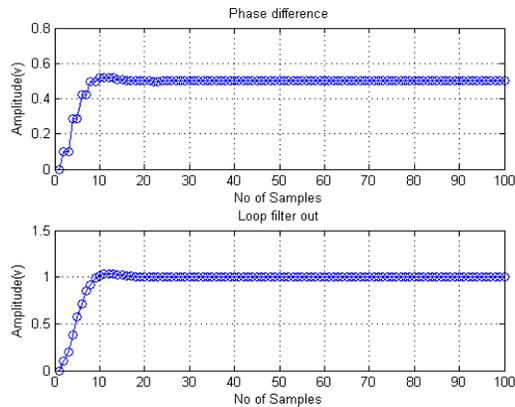
Fig.8. Outputs of Phase Detector and Loop Filter
