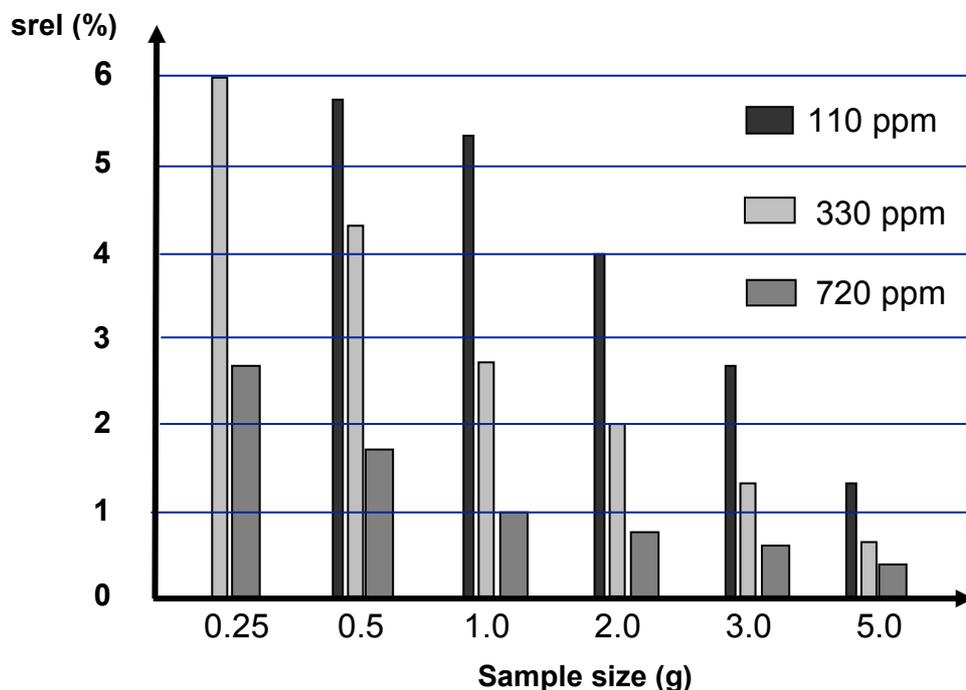
In both cases, with decreasing sample size the relative standard deviation srel becomes worse. Therefore, it is necessary to use the optimum sample size in order to achieve precise results. A good repeatability is achieved the sample size is increased particularly for low water content values.
