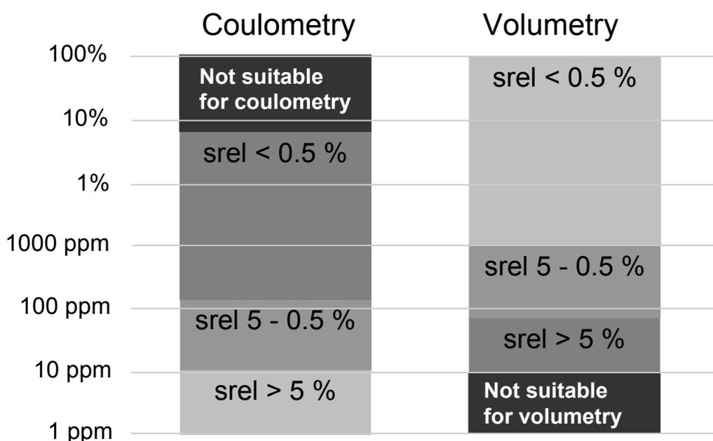
In the following graphs, the relative standard deviation  $s_{rel}$  (%) of several series with different water content are given as a function of the sample size:
