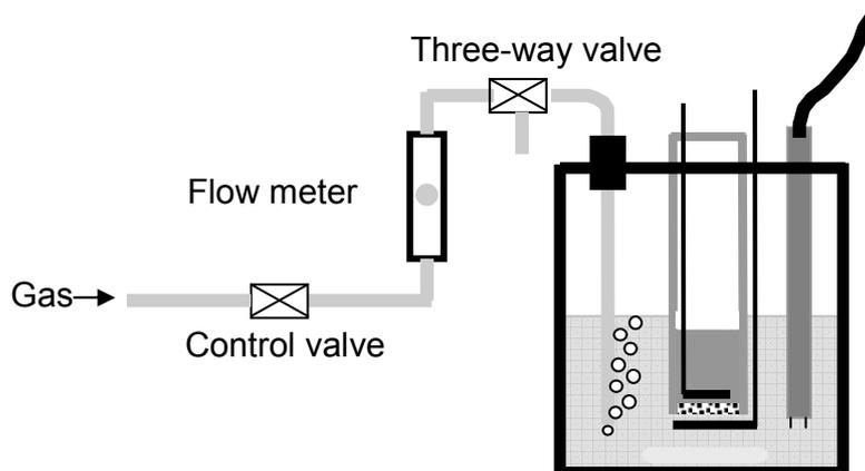
The flow rate has to be constant to determine the volume necessary to calculate the water content:  $\text{gas volume} = \text{gas flow rate} \times \text{time}$ .
