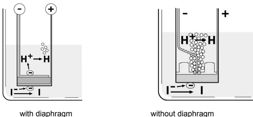
The first commercially available diaphragmless cell for KF coulometry was introduced in 1989. The main advantages compared to cells with diaphragms are:
