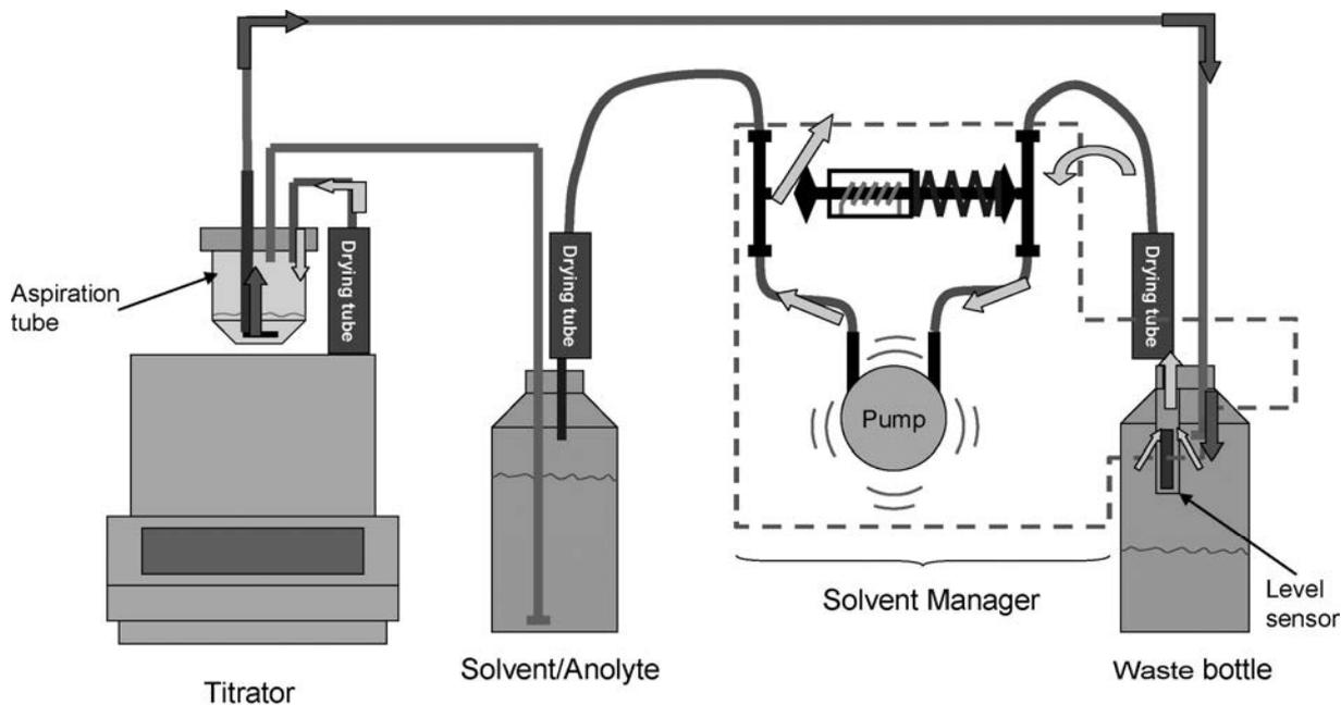
Step 2: The Analyte is drained into the waste bottle by applying vacuum.
