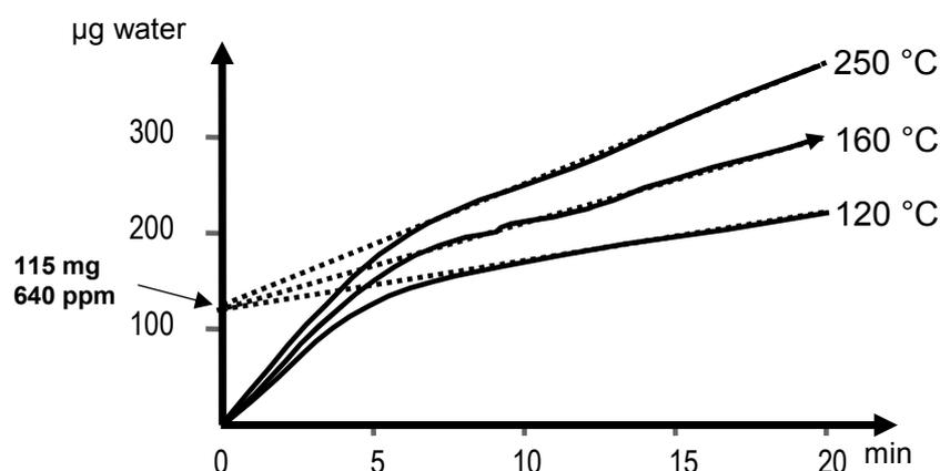
The determination was carried out for a period of 20 minutes (max. time) with the drying oven set to 120 °C, 160 °C and 250 °C. The following results were obtained:
