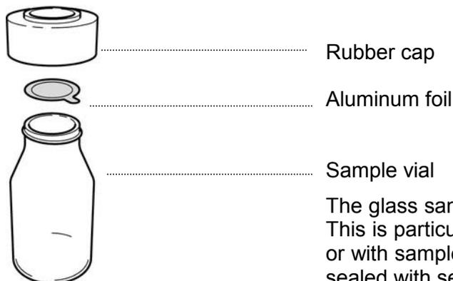
The glass sample vials have a large volume (up to 25 mL). This is particularly important with light samples (e.g. fibers) or with samples of low water content. The sample vials are sealed with self-sealing aluminum foil and a rubber cup.
