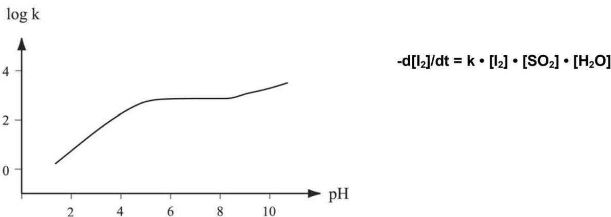
One possible explanation for the influence of pH on the reaction rate is that it is not the sulfur dioxide itself that is oxidized by iodine under the influence of water, but rather the methyl sulfite ion. This is formed from sulfur dioxide and methanol according to the equation:
