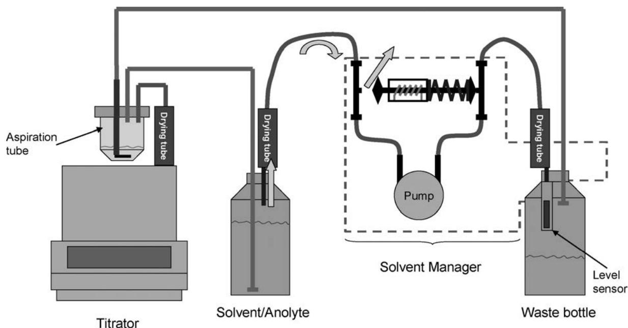
Step 4: After a predefined time or by manual interaction the pressure within the solvent/anolyte bottle is relieved by switching the magnetic valve into the initial position.
