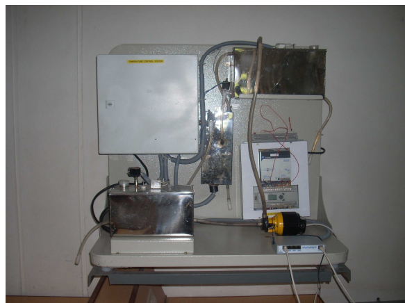
Fig 1.1 Photographic view of real-time experimental pilot plant with LCU and GPRS Gateway device
